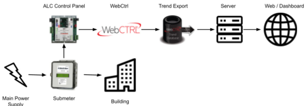
Fig. 7. Block Diagram showing the path of demand data through WebCtrl.
