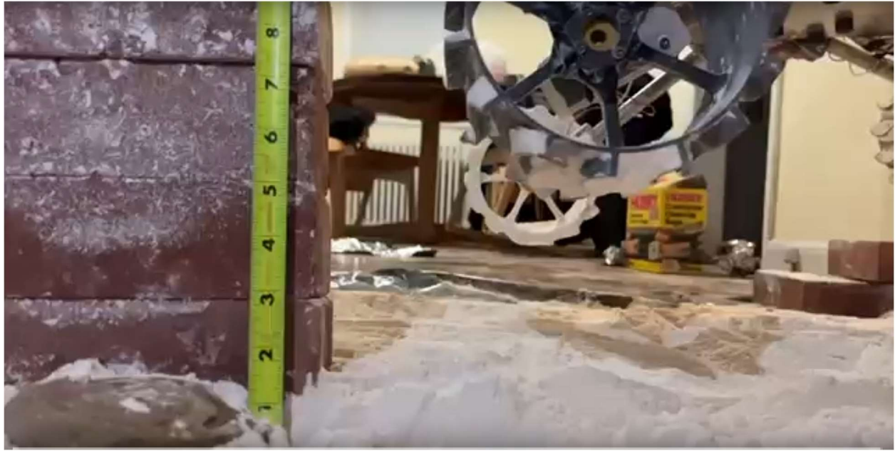
Figure 52: Setup of the drop test conducted on the micro rover to test its survivability of deployment on the Moon.
