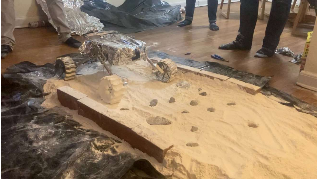
Figure 49: Setup of secondary drivetrain test where the micro rover will traverse small rocks within the flour mimicking lunar dust.
