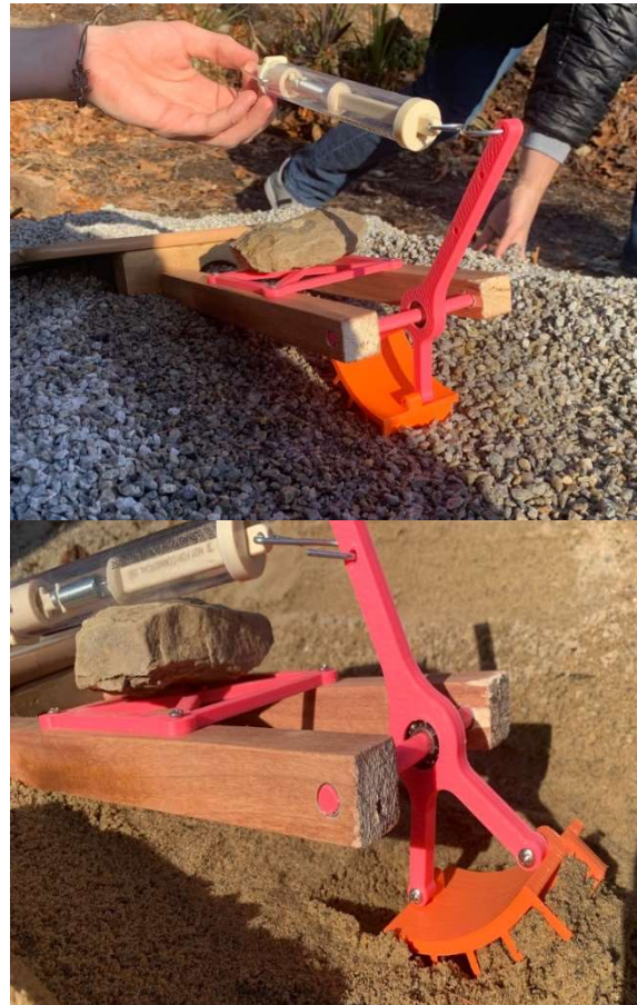
Figure 46: Testing rig designed for measuring the torque of various tread designs in different sizes of gravel.
