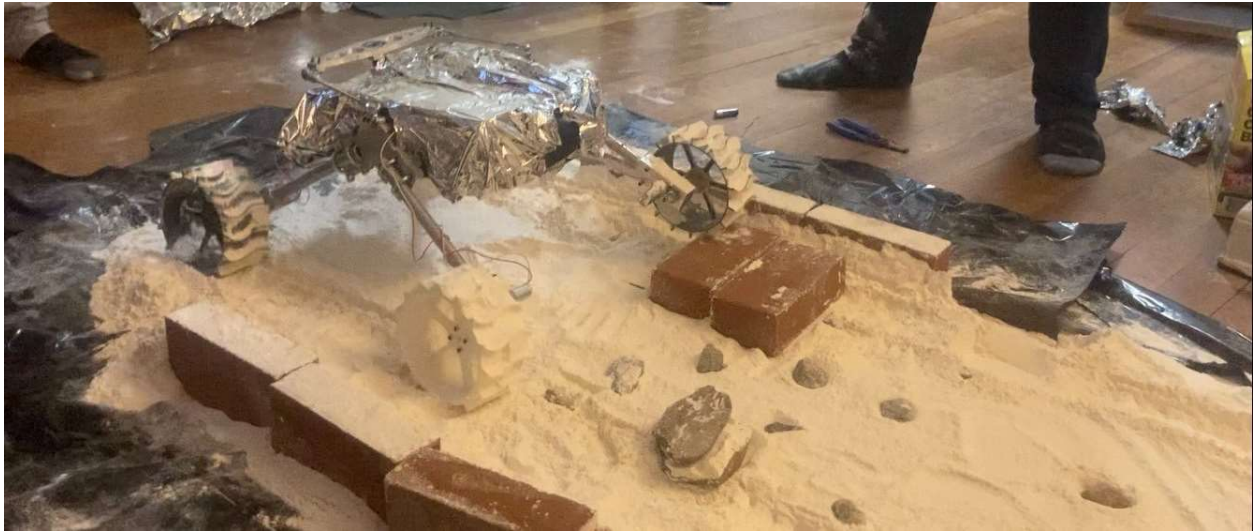
Figure 51: Setup of tertiary drivetrain test where the micro rover is to climb over bricks on the side, while the other side will have to climb over stacked rocks placed within the flour mimicking lunar dust.
