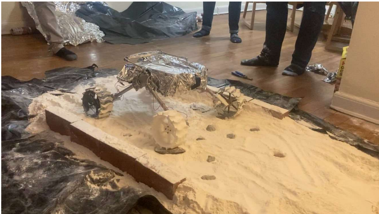
Figure 50: The micro rover navigating the secondary drivetrain test mid-traversal over a small rock.
