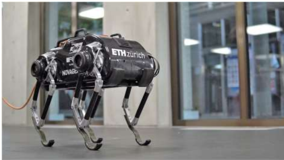
Figure 5: An image of ETH Zürich's rover called Spacebok.
