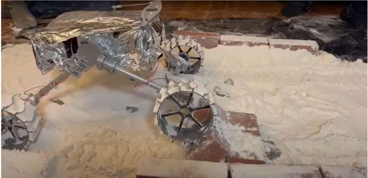
Figure 53: The micro rover climbing up an incline made from bricks to test the drivetrain’s torque and grip when climbing.
