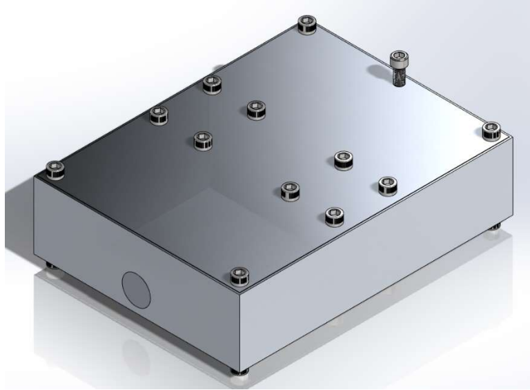
Figure 55: Modified chassis CAD model for the use of thermal simulations within Ansys Workbench 2022.
