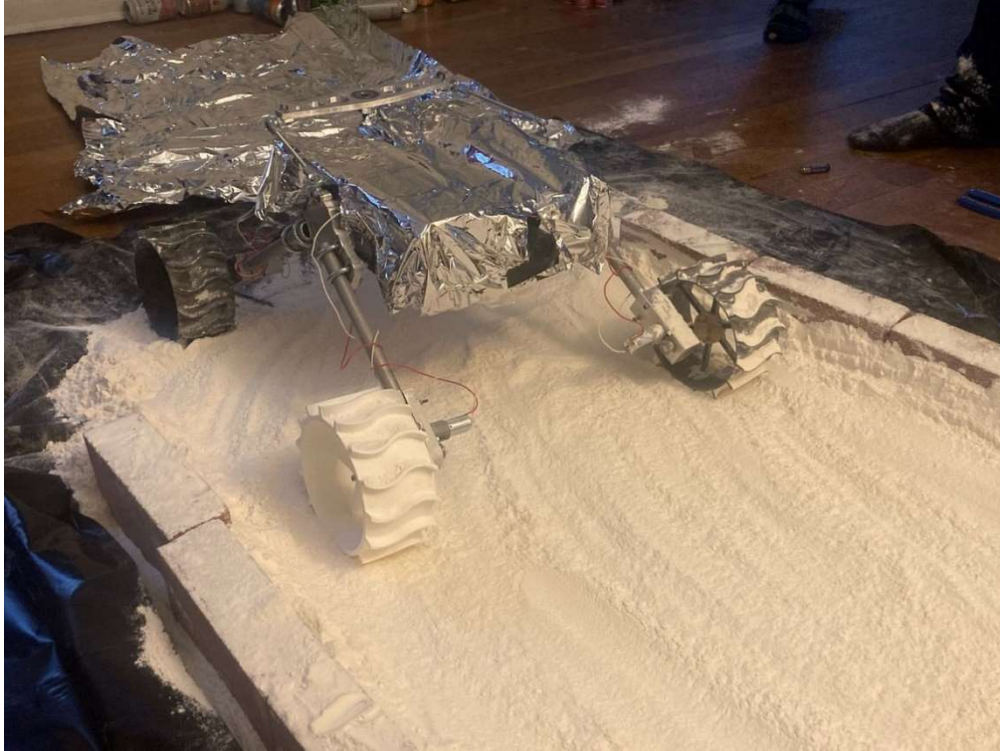
Figure 48: Setup of initial drivetrain test where the micro rover drives forward in the flour mimicking lunar dust.
