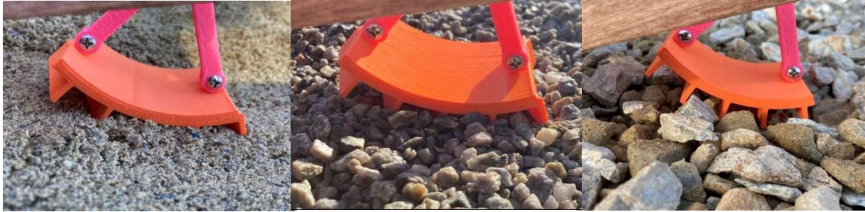
Figure 47: Example of a tread design’s torque being tested in 3 varying sizes of gravel.
