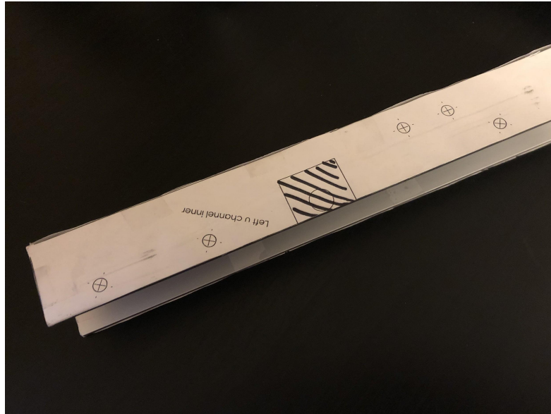
Figure 41: 6061 aluminum alloy U-shaped cart frame
