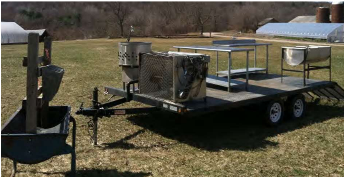
Figure 6: Open-air MPPU with the kill cones on the left, and scalder and plucker centered (Anderson and Hashley, 2012)
