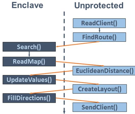
Figure 23: ECALL/OCALL Interfaces without Reduction
