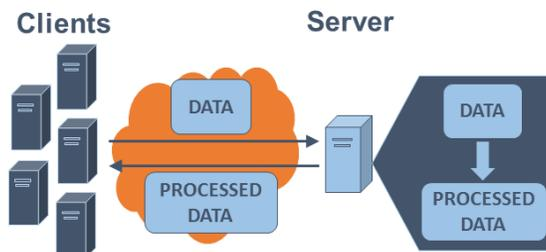
Figure 1: Client-Server Web Service Architecture
