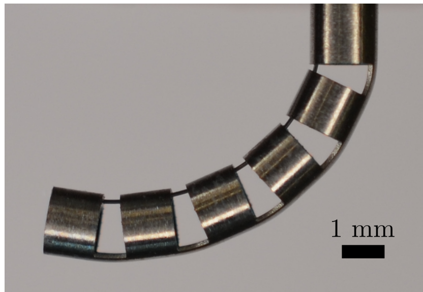
Figure 1.3: An example of notched-tube continuum wrist. These mechanisms are manufactured out of a tube of superelastic Nickel-Titanium (Nitinol) and are articulated by pulling a tendon attached to the tip. Notched-tube wrists can be created in small diameters and can bend in tight radii of curvature. A bending radius of 1.42 mm was demonstrated in [2].
