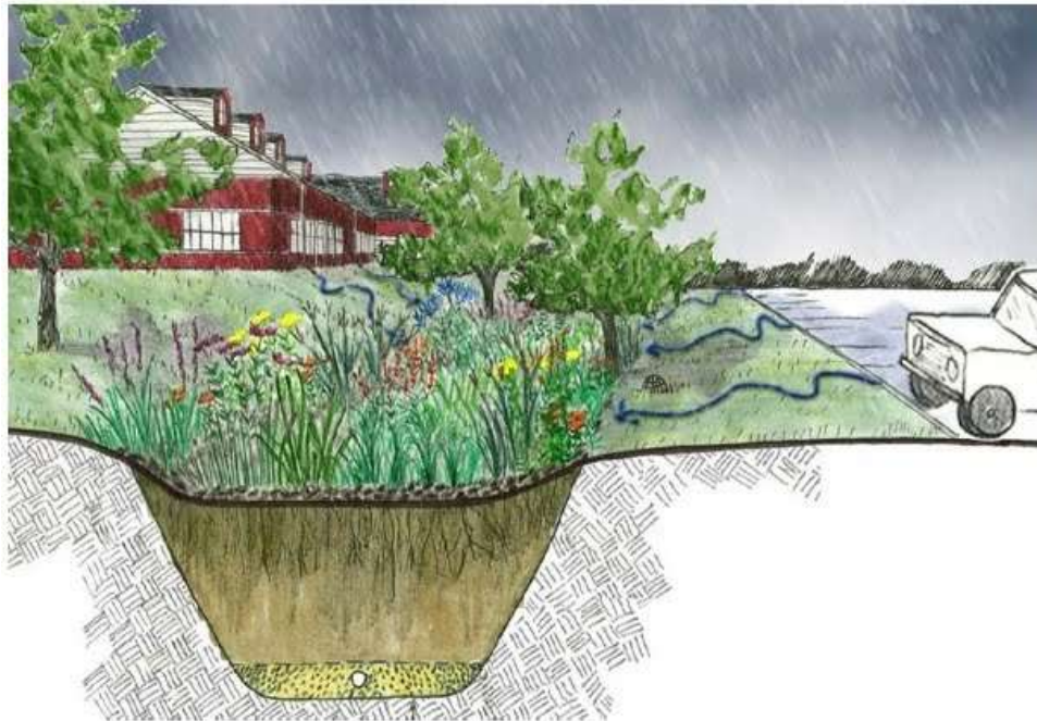
Figure 17. Illustration of a rainwater garden reducing runoff. (Domnik, 2010)
