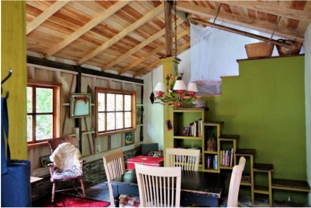
Figure 9. A staircase with built-in storage.
