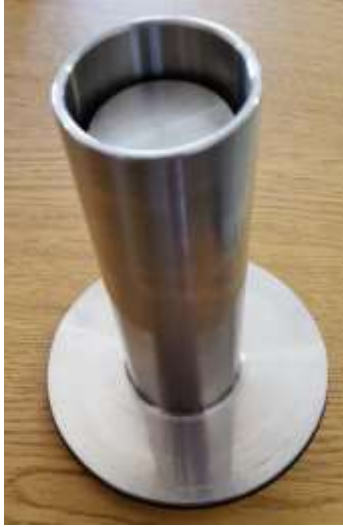
Figure 86: Photograph of the test cell for conductivity and permittivity measurement
