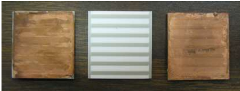
Figure 105: Photograph of the top surfaces of test samples; left (fast copper-plated nano-textured surface) middle (bare surface) and right (slow copper-plated nano-textured surface)
