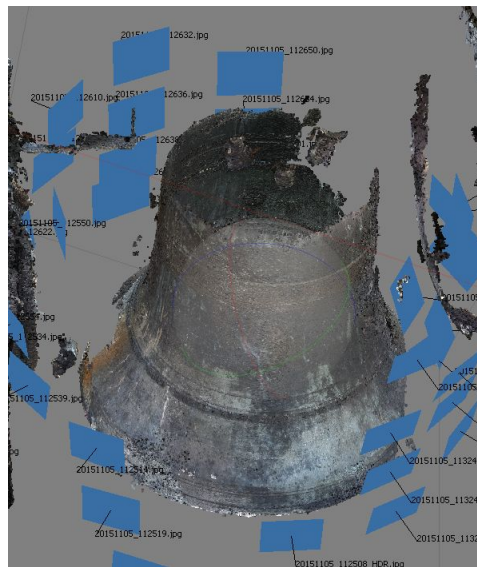
Figure 27: Assembled dense point cloud of a bell
