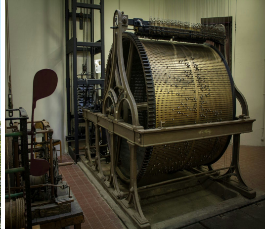
Figure 5.2: Roller with striking pins 29
