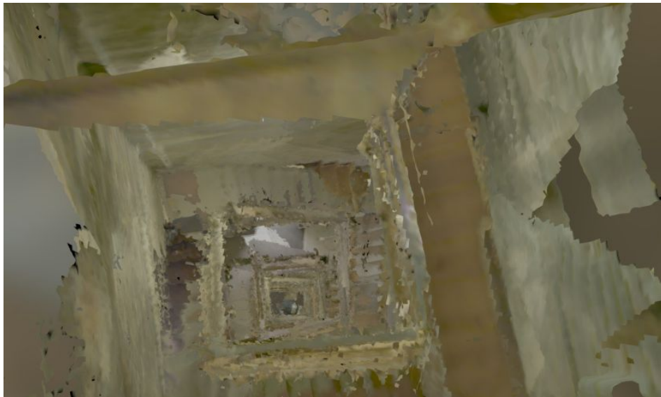
Figure 23: Rendered color mesh of the San Giovanni Grisostomo Bell Tower using Project Tango. View looking down into the shaft with staircases around the perimeter.
