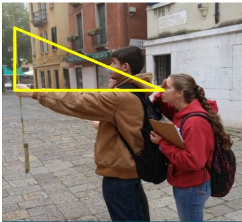
Figure 22: Creating triangle from observer to tower in determining height. 73
