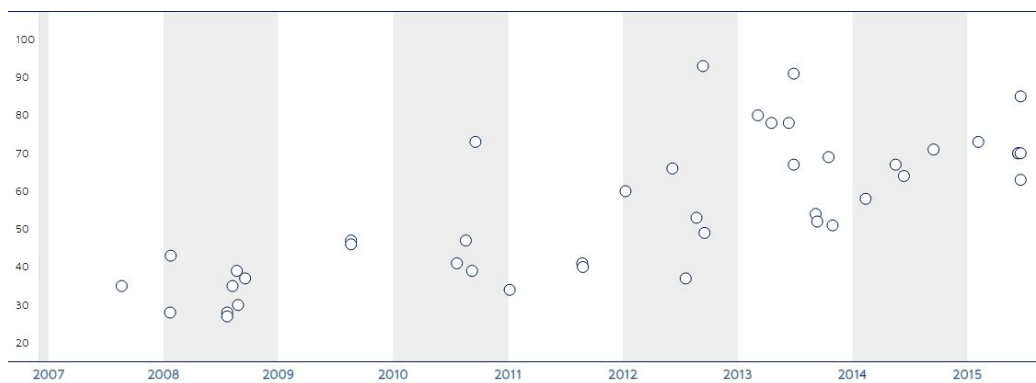
Camera benchmark scores over time. Benchmark measures color recognition, exposure range, and usable ISO levels 97
