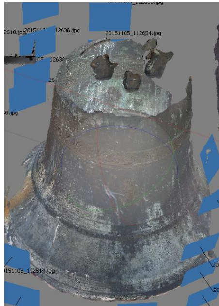
Figure 28: Textured model of a bell created with PhotoScan
