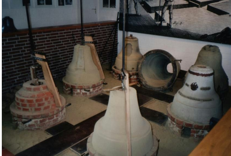
Figure 3: Bell casting molds 20
