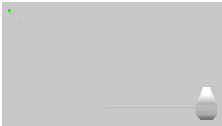
Figure 5.10: Paths generated with A* usually do not follow a straight line from the source to the destination even when all cells are marked as unoccupied.
