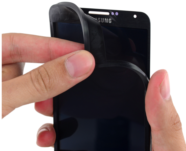
Figure 30: The DK2 screen removed from the device [12]
