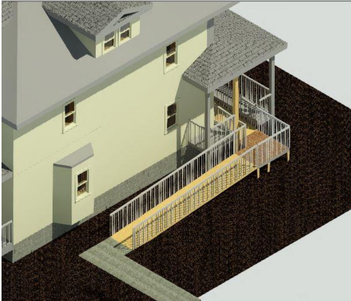
Figure 35. Rendering of the first floor accessibility ramp
