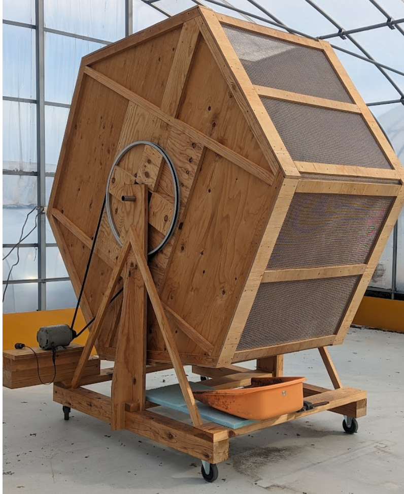
Figure 10: A large-scale wheel whose design was inspired by coffee bean rotary driers. This machine has the potential to reduce significant labor in drying and sifting through indigo leaves entirely manually.
