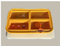
Figure 44: The casting process for the gelatin phantoms used for testing tissue density detection.
