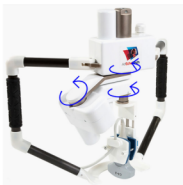
Figure 9: Image of the Estelle teleoperated ultrasound system. (ESTELE, Robosoft Engineering, Anglet, France) When in use a surgical assistance positions the robot by use of the black frame, while a surgeon can teleoperate the marked degrees of freedom.
