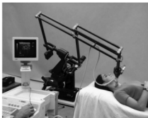
Figure 7: Image of early robotic ultrasound system developed by Abolmaesumi et al. for ultrasound scanning of the carotid artery [4].
