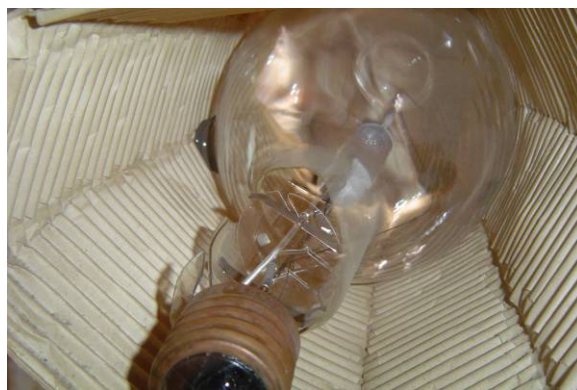
Figure 6: Image showing an example of a broken HID lamp in ESPH's warehouse A
