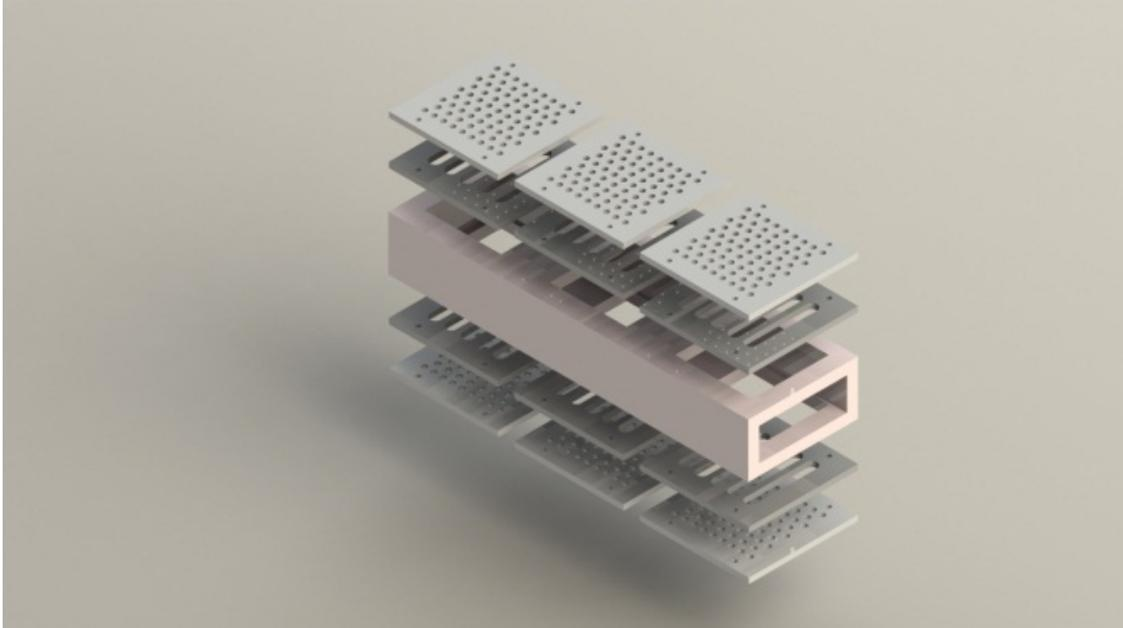
**Figure 46: 50cm<sup>2</sup> Active Area Stack Exploded**
