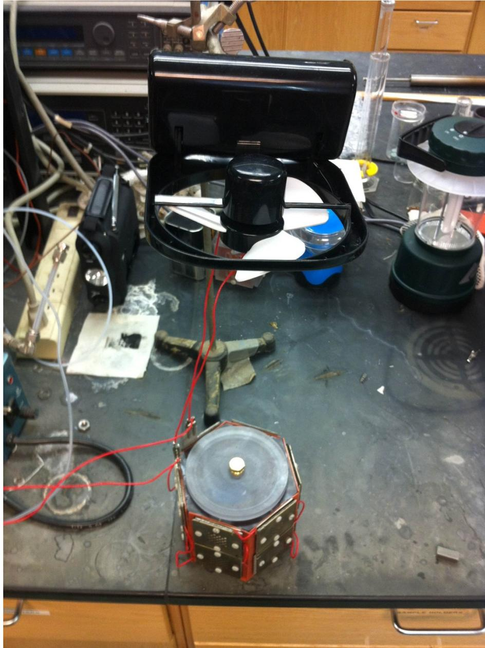
**Figure 19: Fan Powered by the Fuel Cell Stack as an Ancillary Utility**
