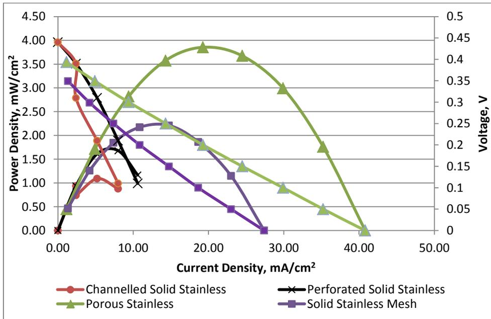
Figure 22: Effects of Cathode C.C. on Performance (Single Cell PDMFC, MeOH Gel)
