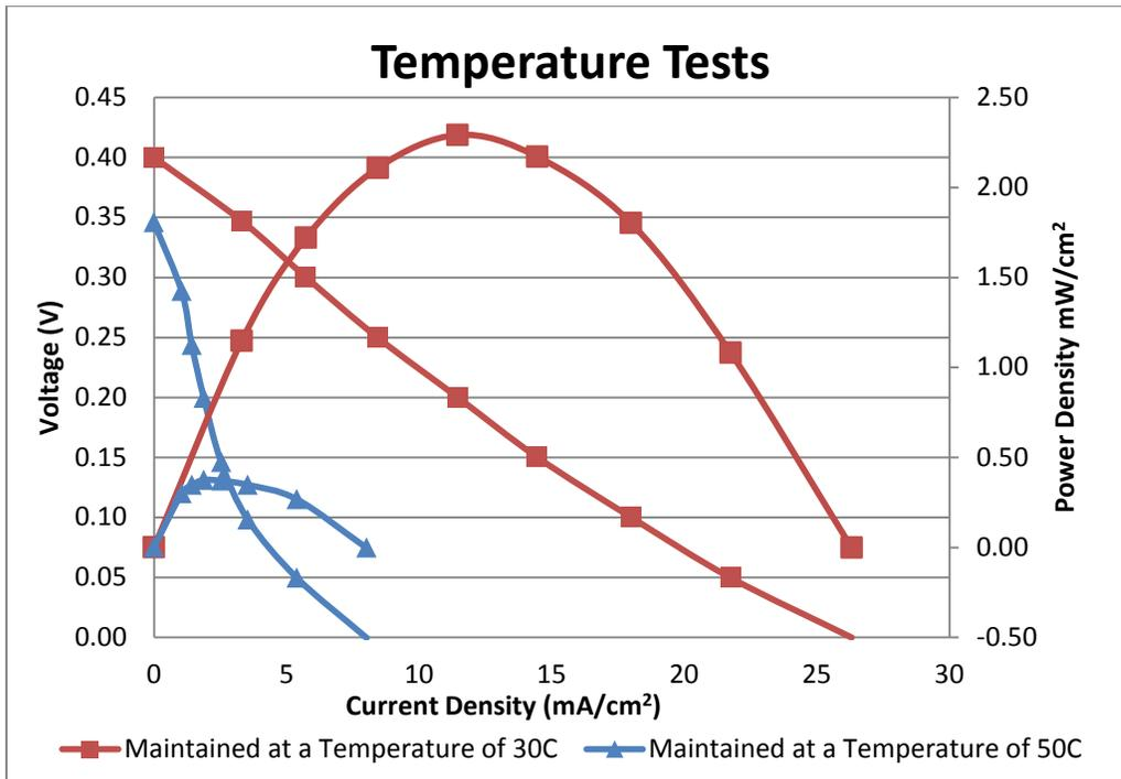
Figure 25: Temperature Test Results (Single Cell, IRD MEA, MeOH Gel)
