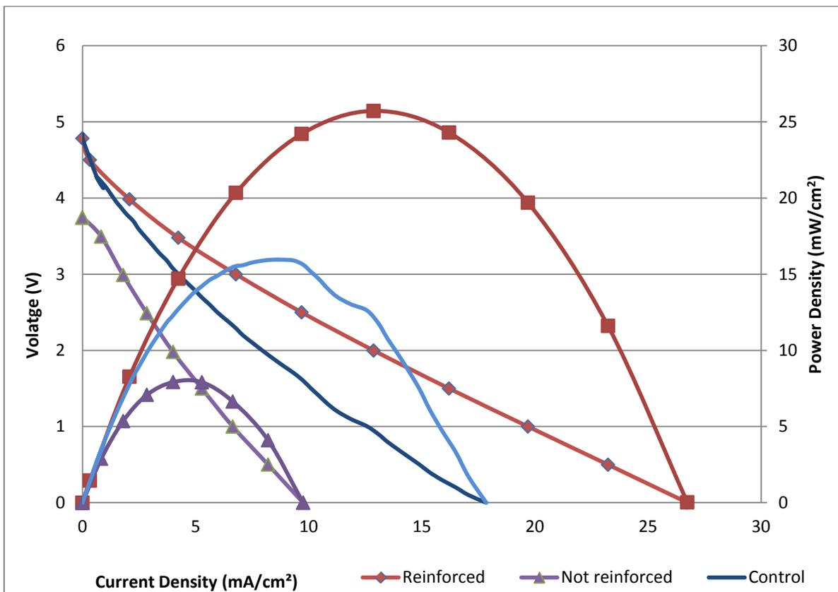
Figure 31: Reinforcement Techniques on Current Collectors (Stack Layout, MeOH Gel Fuel)
