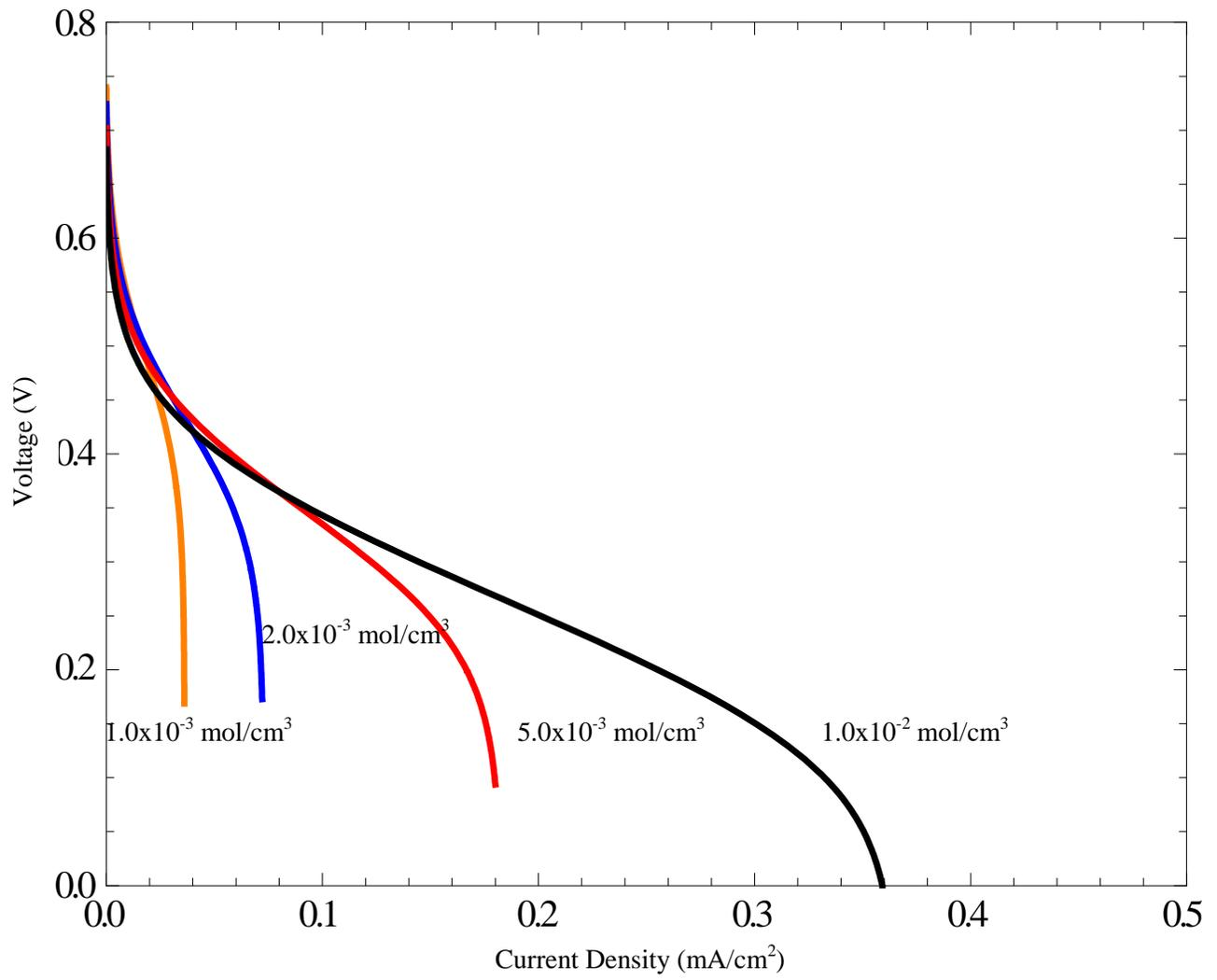
Figure 44: MeOH Bulk Concentration in PDMFC Model Polarization (303K, MT Coef:  $1.0 \times 10^{-4}$ )
