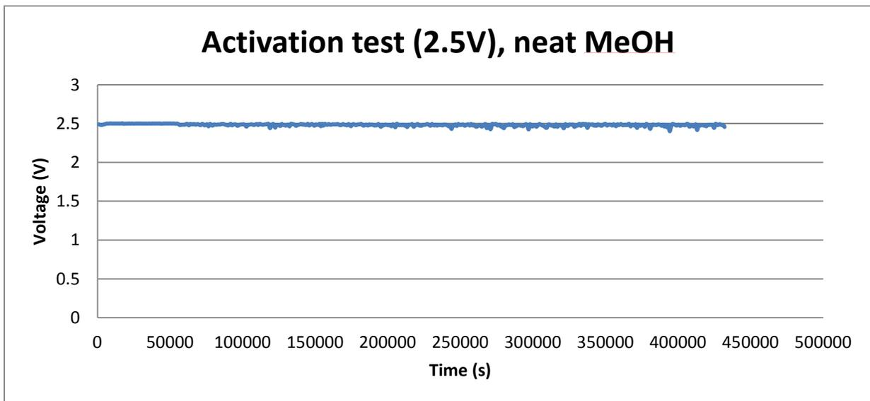
**Figure 32: 5 Day Activation Test (Optimized Current Collector Stack Layout, Neat MeOH Fuel)**
