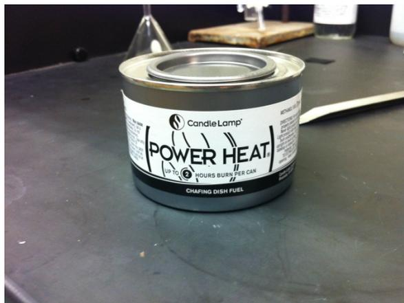
**Figure 6: Methanol Chafing Fuel, Power Heat Brand, Similar to Sterno**
