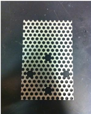
**Figure 11: Wire Mesh Current Collector**
