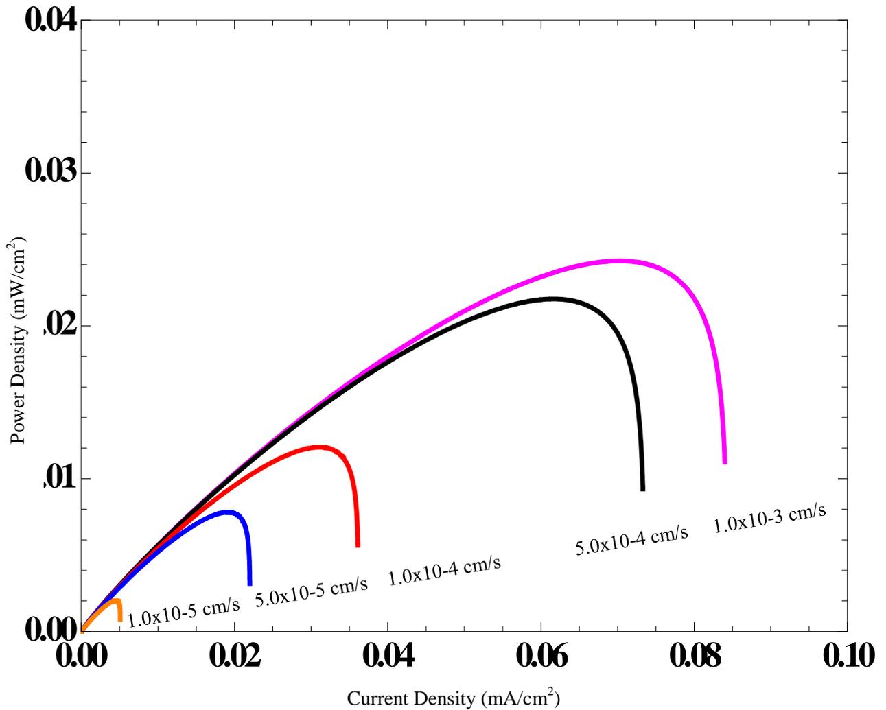
Figure 43: Mass Transfer Coefficient Variable in PDMFC Power Graph (303K, 1.0M)
