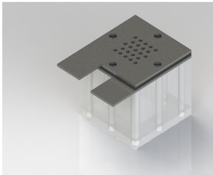
**Figure 5: Single Cell Schematic Compacted, 5cm<sup>2</sup> Active Area**
