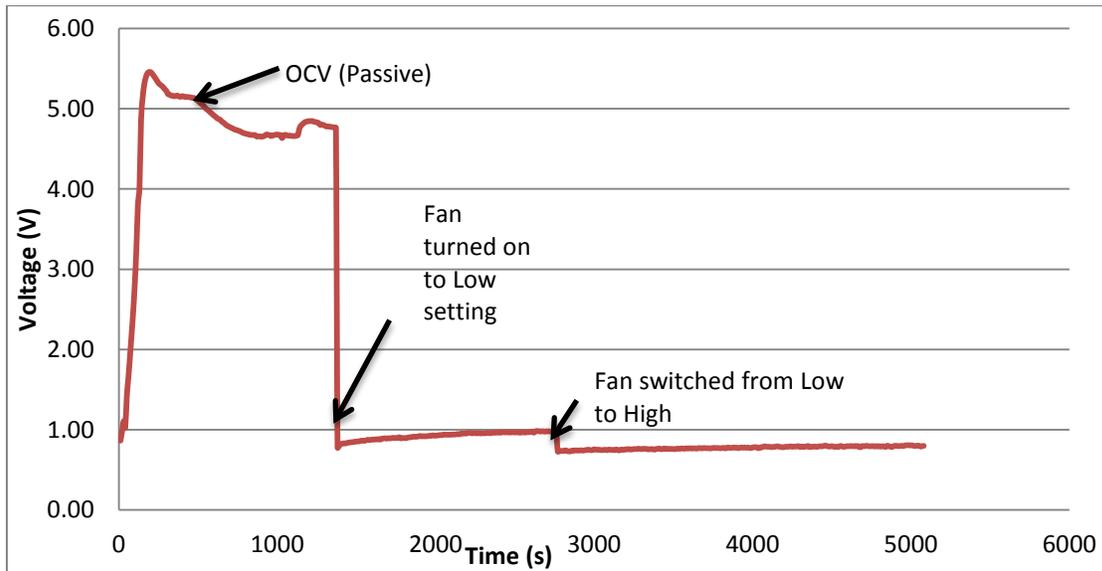
Figure 38: Active vs. Passive (Optimized Stack Layout, 25g MeOH Gel Fuel)
