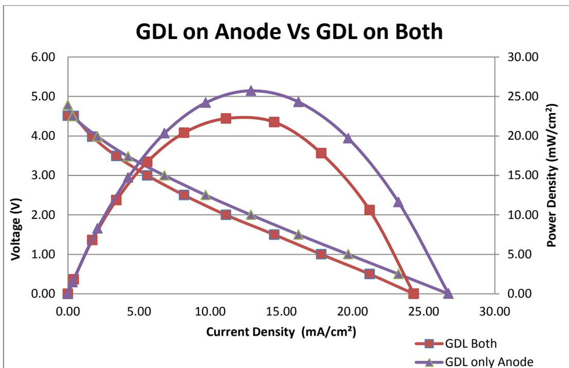
Figure 28: Gas Diffusion Layer Presence Results (Stack Layout, MeOH Gel Fuel)
