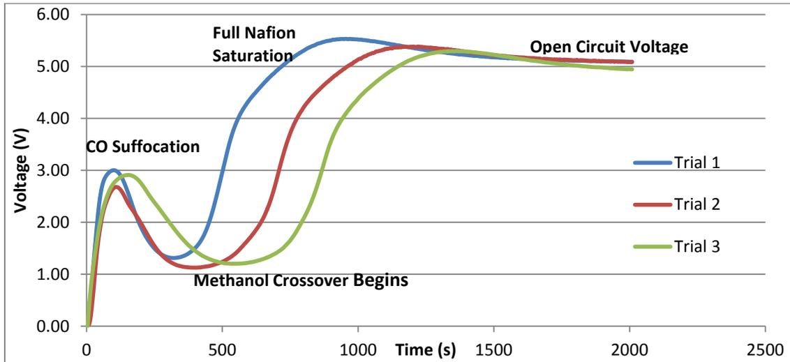
Figure 27: Initial Fuel Injection Results (Stack Setup, 25g MeOH Gel)
