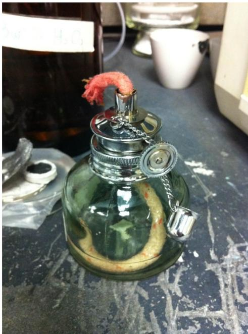
**Figure 36: Neat Methanol with Adjustable Wick**
