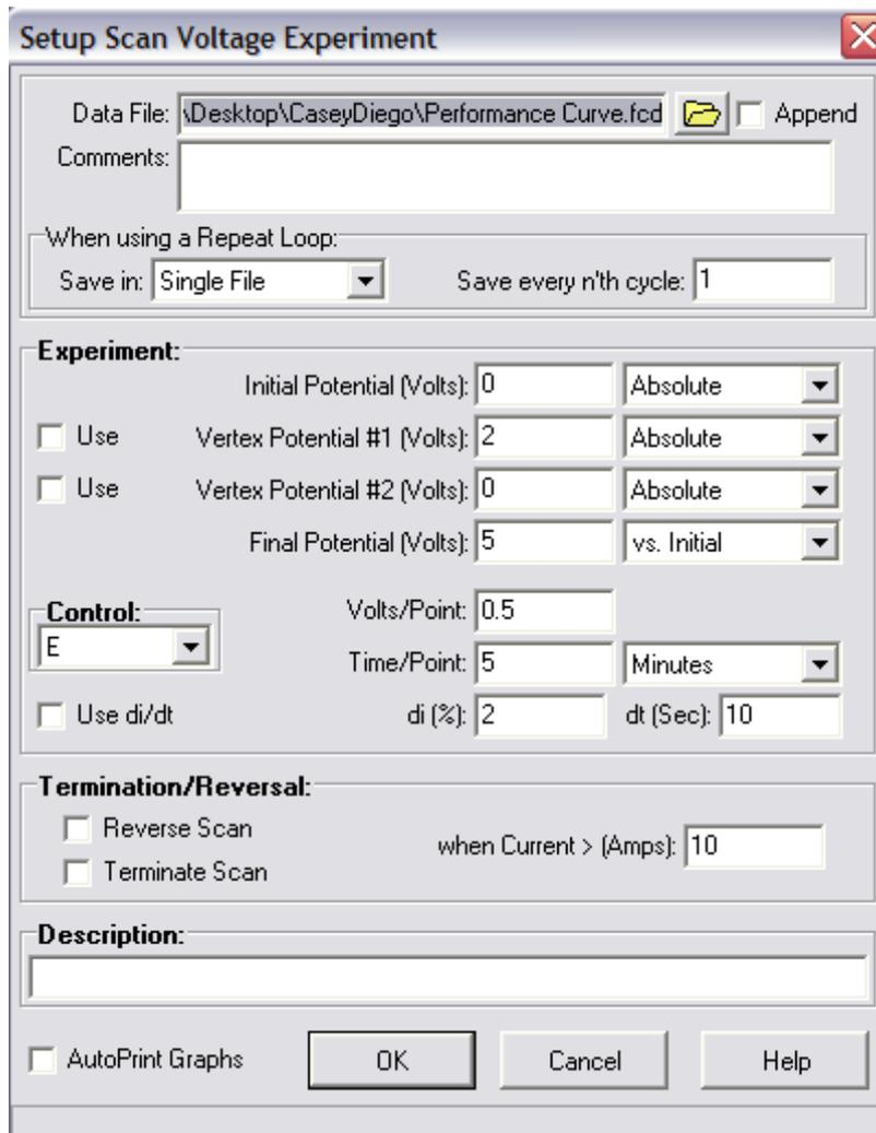
Figure 16: Input Used to Run Voltage Scan Tests on Fuel Cell
