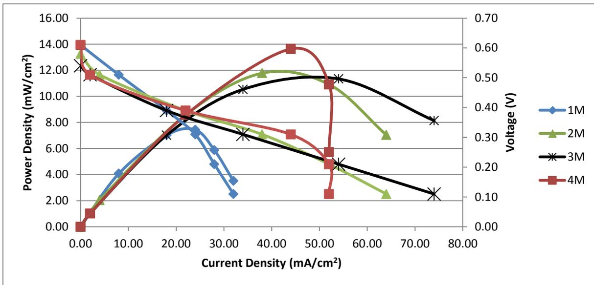
Figure 21: Liquid MeOH Solution with Diff. Concentrations (Single Cell PDMFC, IRD MEA)
