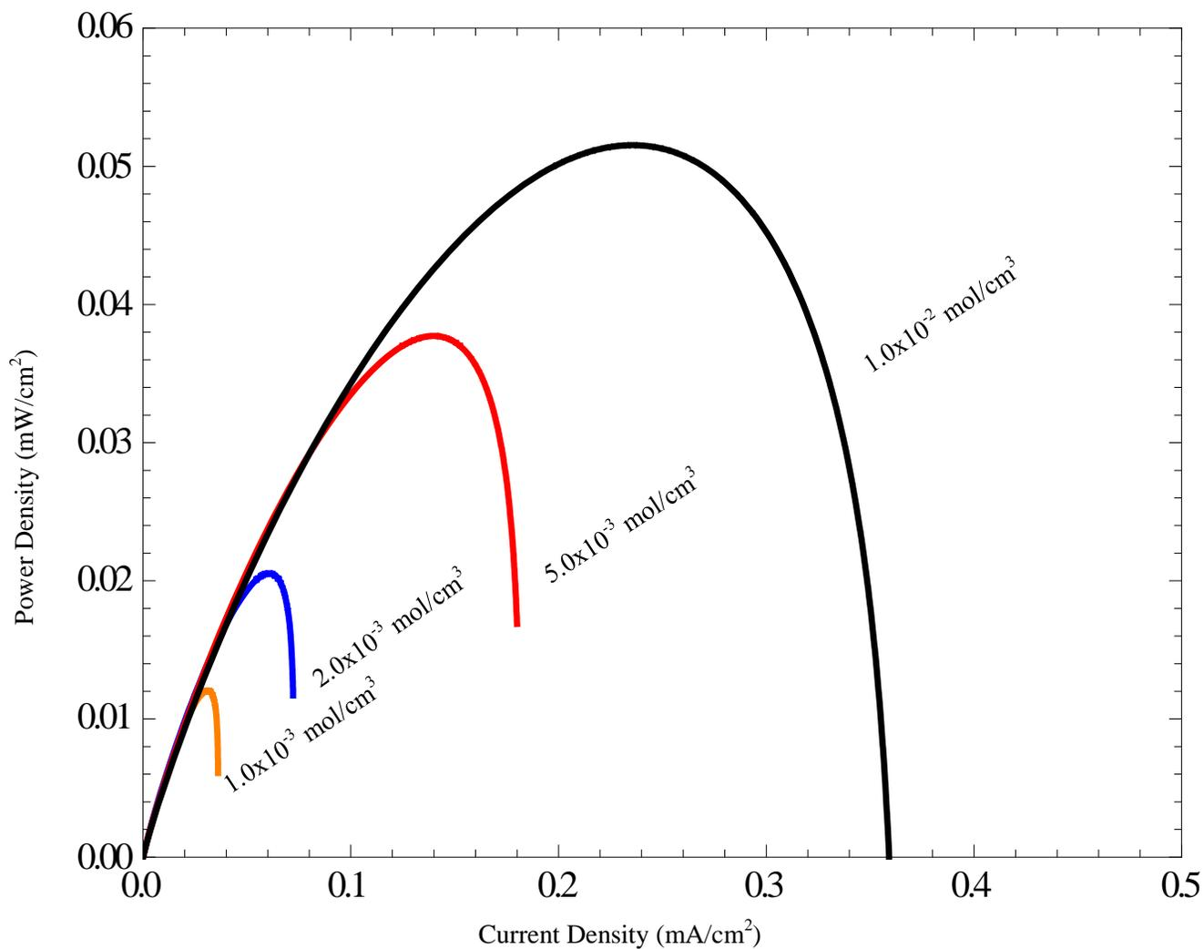
Figure 45: MeOH Bulk Concentration in PDMFC Model Power Graph (303K, MT Coef:  $1.0 \times 10^{-4}$ )
