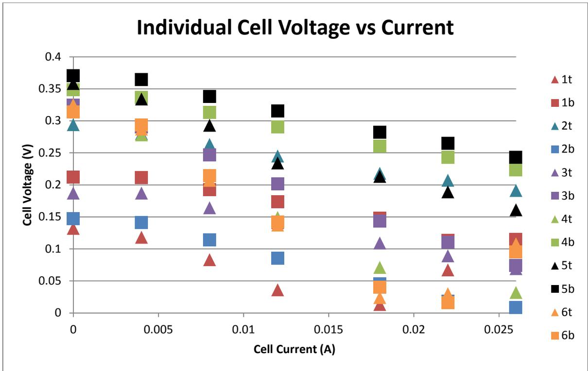
Figure 30: Individual Cell Performance by Stack Location (Stack Layout, MeOH Gel Fuel)
