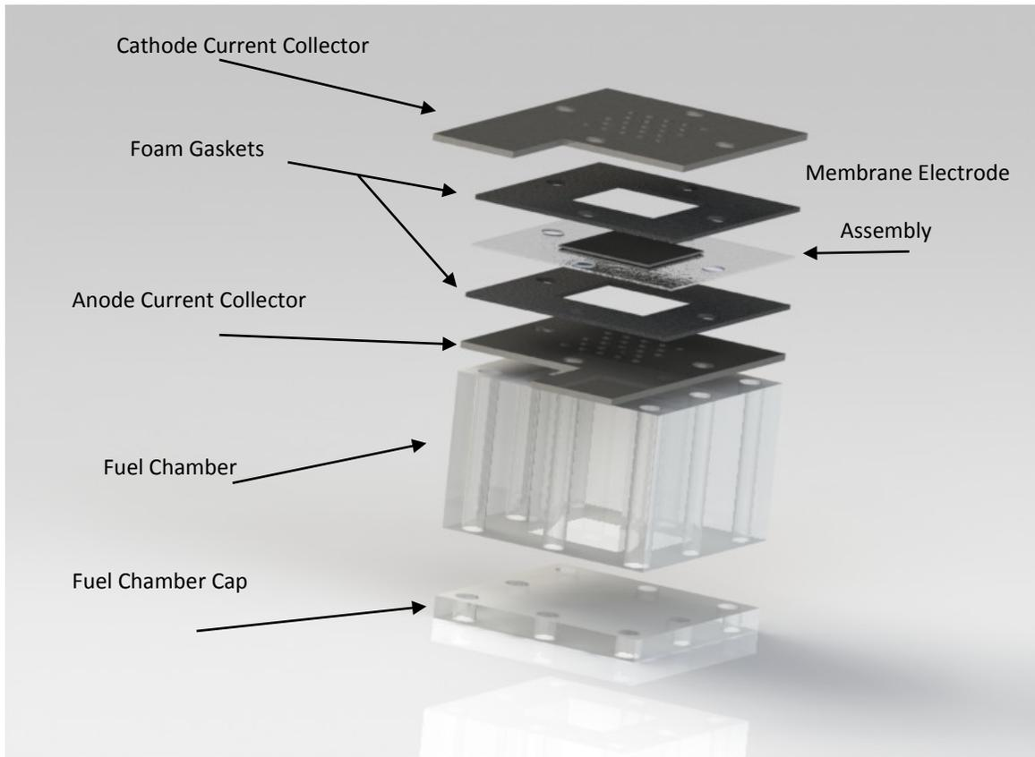
**Figure 4: Single Cell Schematic Exploded, 5cm<sup>2</sup> Active Area**
