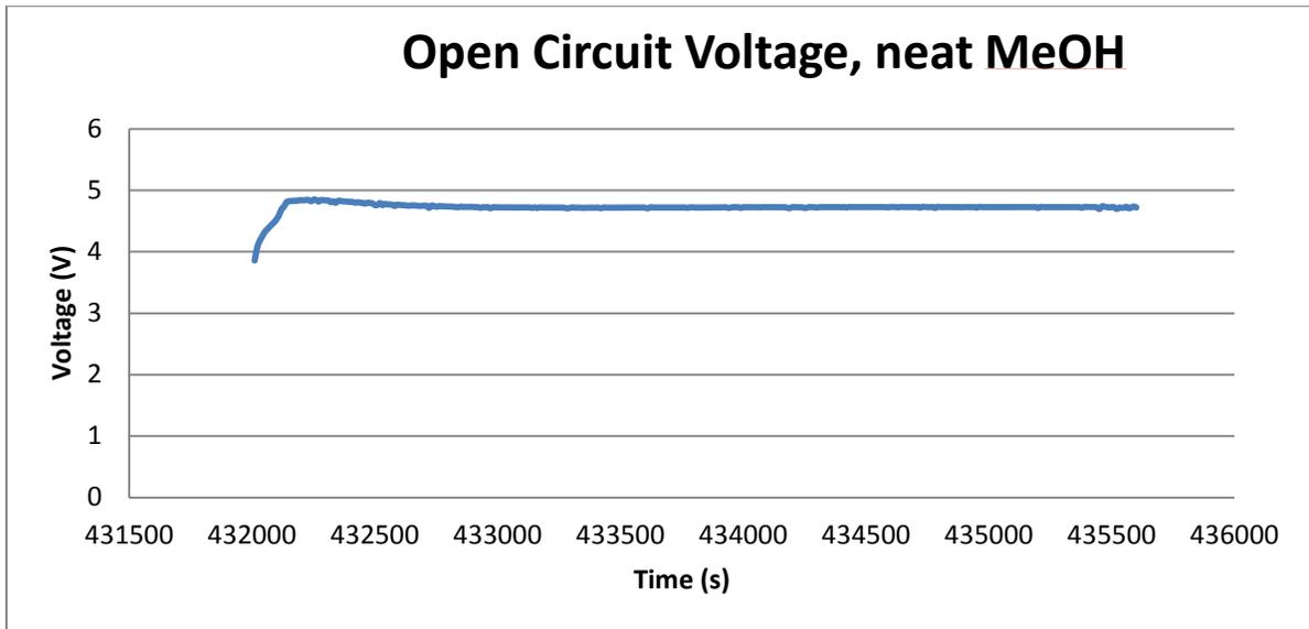
Figure 33: Open Circuit Voltage (Optimized Current Collector Stack Layout, Neat MeOH Fuel)
