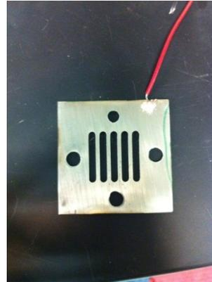
**Figure 10: Channeled Current Collector**
