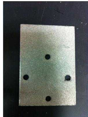
**Figure 12: Porous Current Collector**
