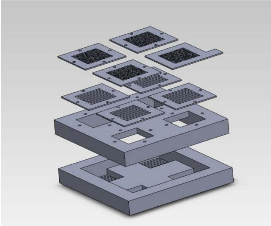
Figure 48: 25cm<sup>2</sup> Stack Exploded
