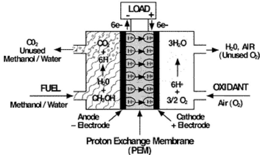
Figure 3: Direct Methanol Fuel Cell Schematic [8]
