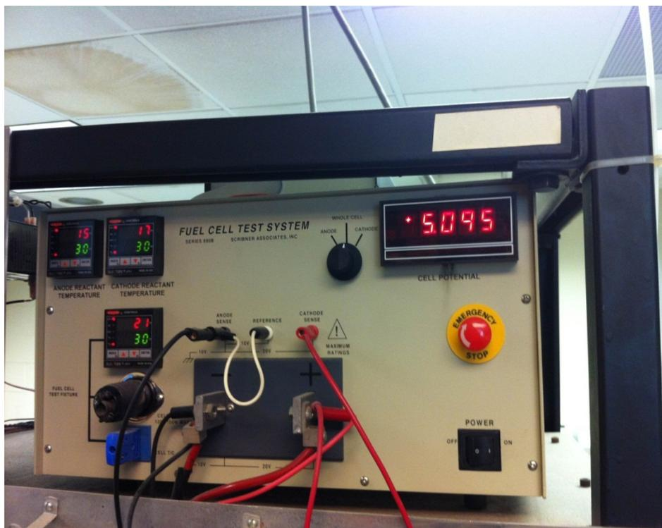
Figure 13: FuelCell Load Box and Display for Test Station
