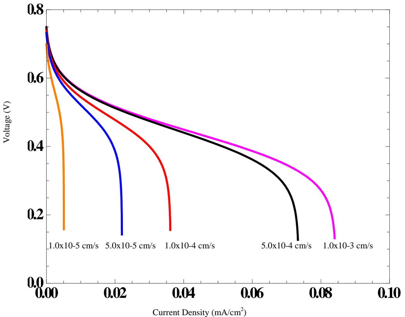
Figure 42: Mass Transfer Coefficient Variable in PDMFC Polarization (303K, 1.0M)
