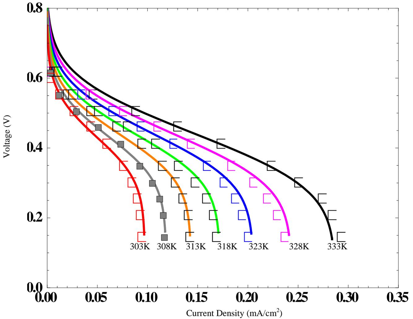
Figure 39: Polarization Plot, 1.0 Molar Solution, variable T. [36]
