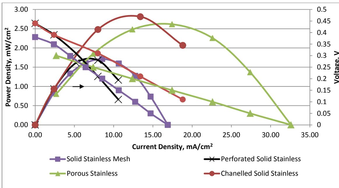
Figure 23: Effects of Anode C.C. on Performance (Single Cell PDMFC. MeOH Gel)
