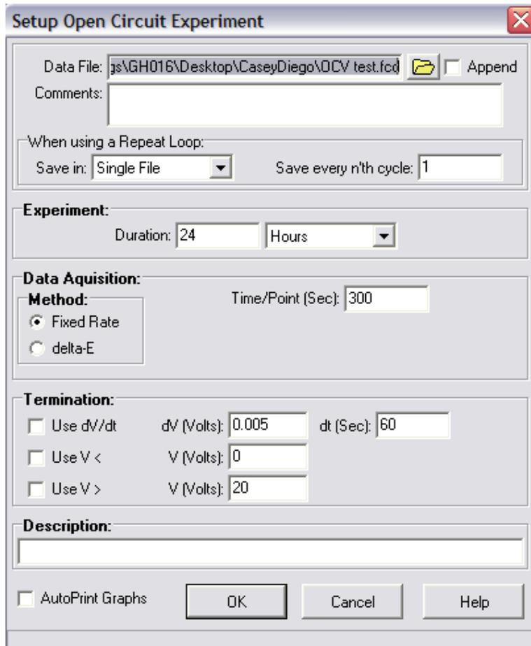
Figure 17: Input Used to Run Long Term Performance Tests on Fuel Cell
