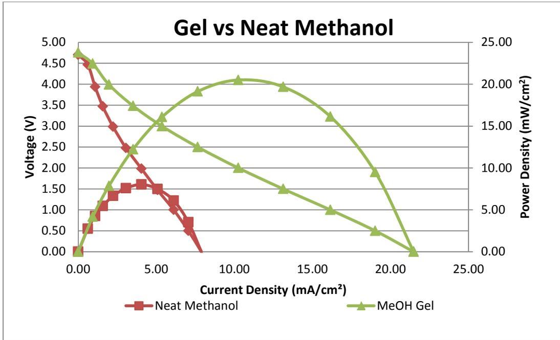
Figure 34: Gel Tests vs. Neat Methanol Tests (Optimized Stack Layout)
