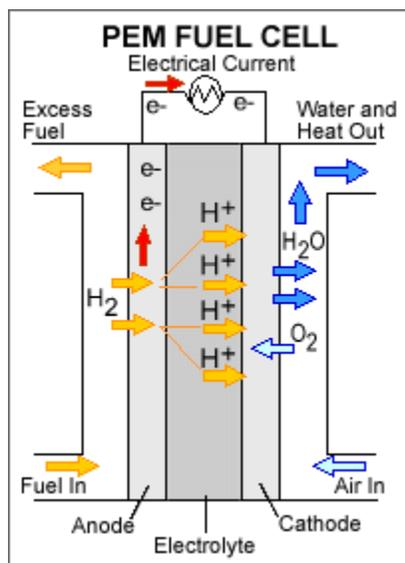
Figure 1: Proton Exchange Membrane Schematic [5]
