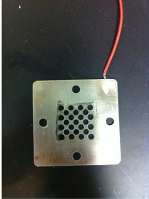
**Figure 9: Perforated Current Collector**
