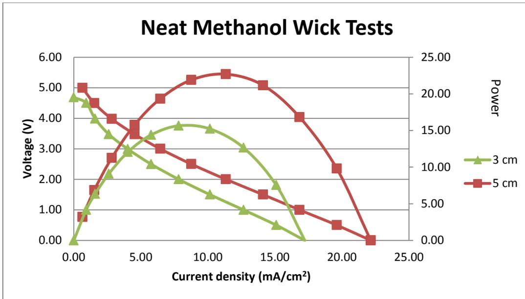
Figure 37: Wick Length Comparison (Optimized Stack Layout, Neat MeOH Fuel)
