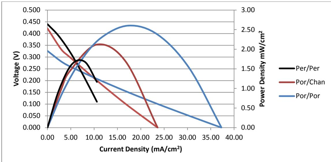
Figure 24: Optimized Current Collector Layout Results (Single Cell, IRD MEA, MeOH Gel)
