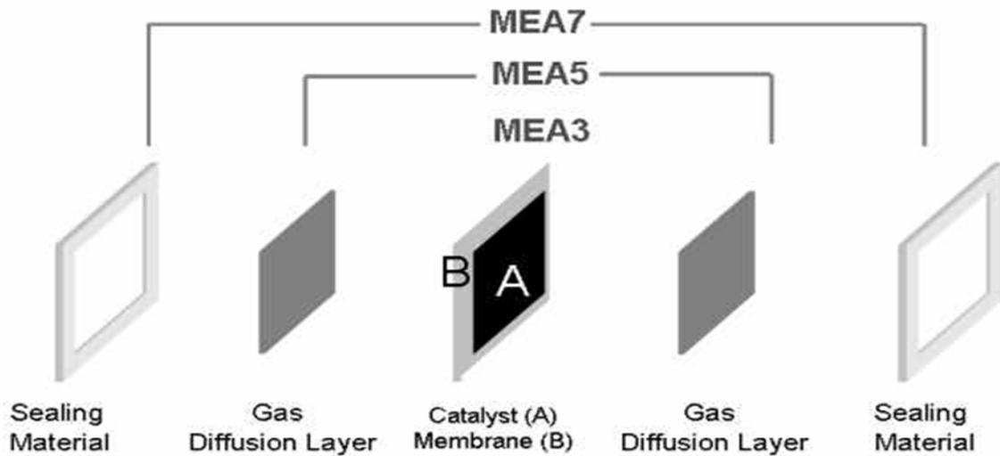
Figure 18: Membrane Electrode Assembly Schematic
