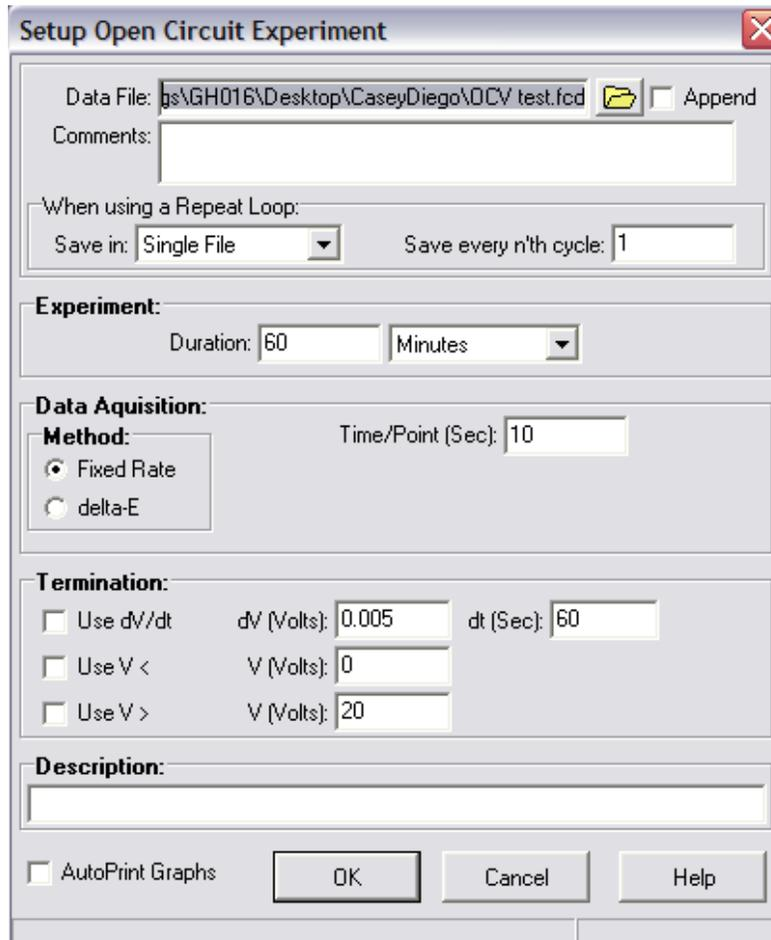
Figure 15: Input Used to Run OCV Tests on Fuel Cell
