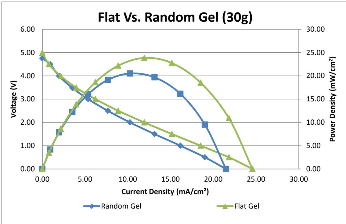
Figure 35: Flat Placed vs. Randomly Placed Gel (Optimized Stack Layout, 30g MeOH Gel Fuel)
