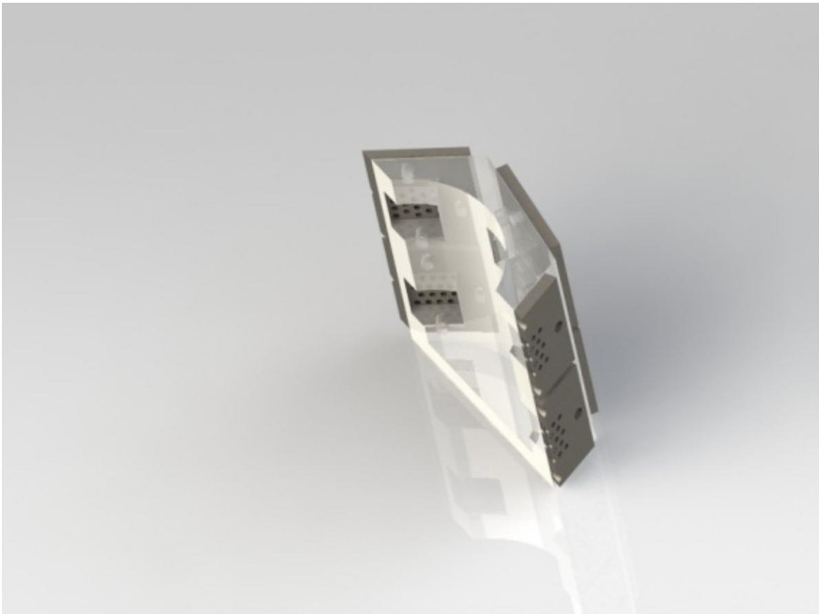
**Figure 7: Cutaway Stack View, 5cm<sup>2</sup> Active Area, 12 Cells in Series**
