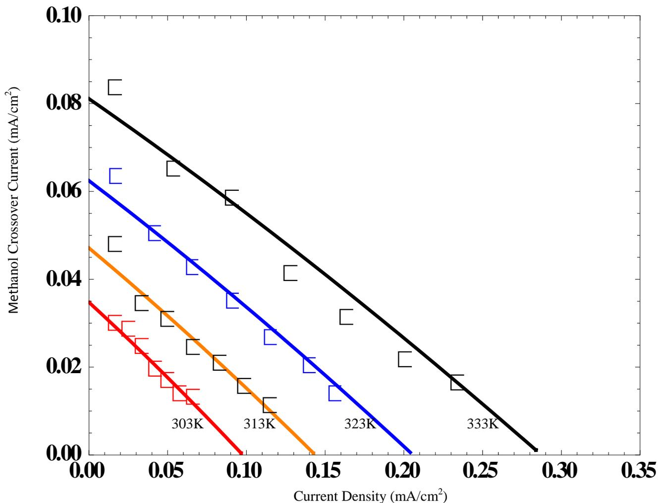
Figure 41: Methanol Crossover Current Density versus Current Density, 1.0M, variable T [36]
