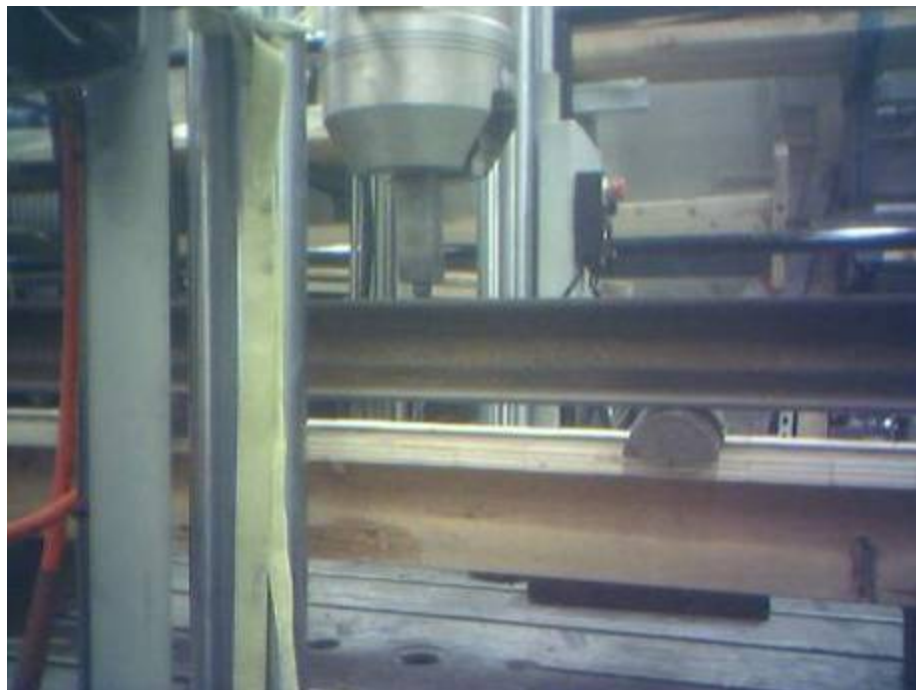
Picture 14: Bend Test – Girder & Plank
