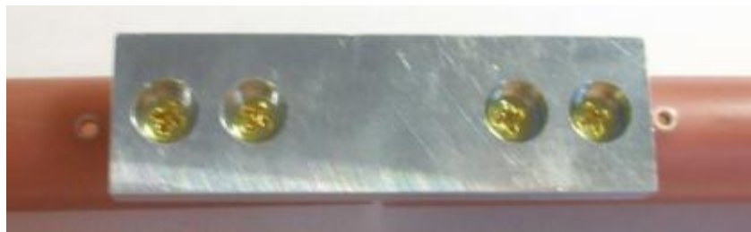
Figure 41: Control Sample of Non-Locking Screw and Plate System in Long Bone Analog
