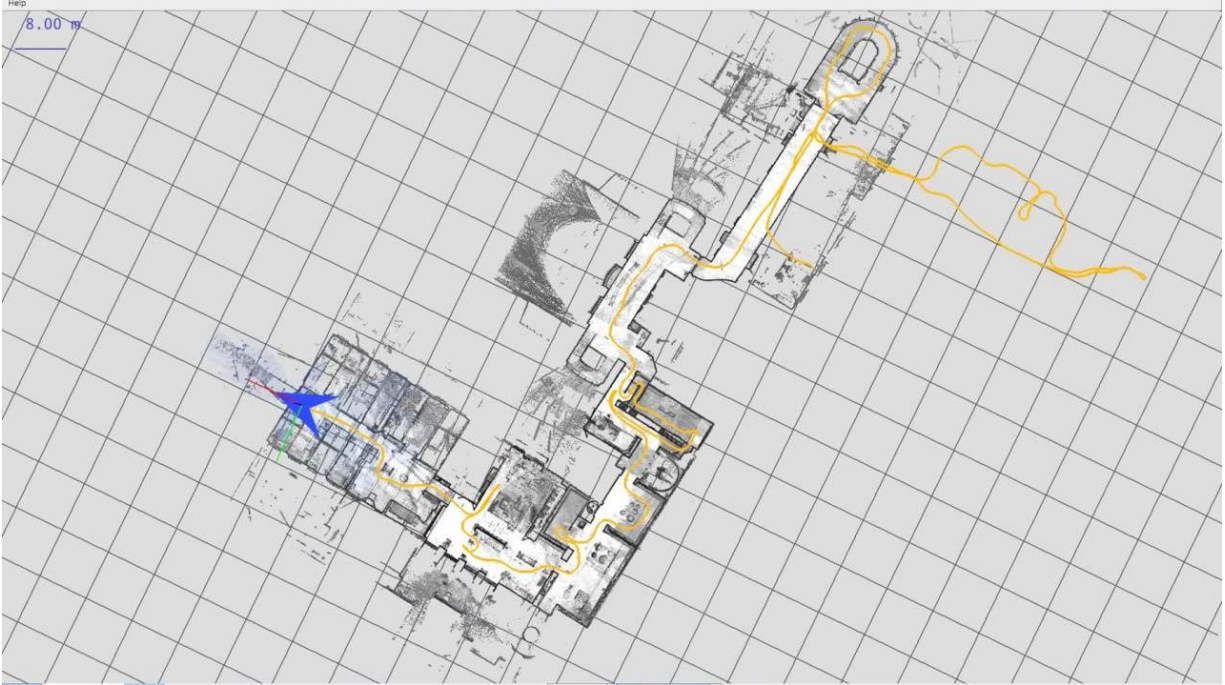
Figure 6: A model of a building produced using LIDAR data and Google Cartographer. (Google Cartographer 2017)
