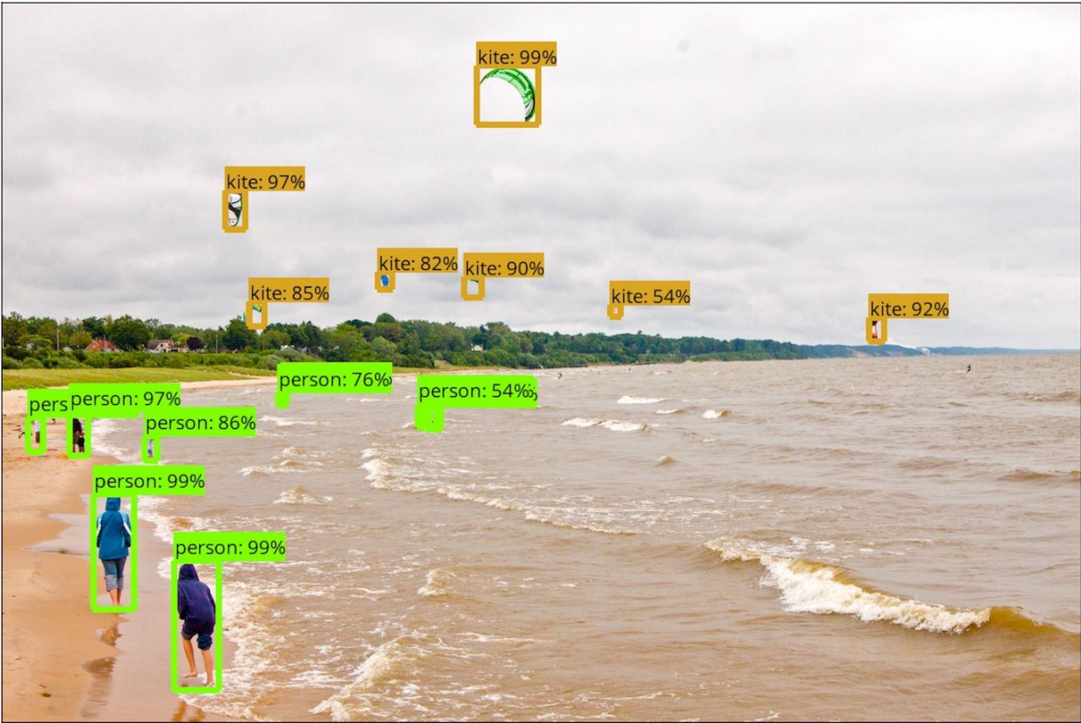
Figure 5: An example of Tensorflow-created labels superimposed on the processed image. (Huang et al. 2017)
