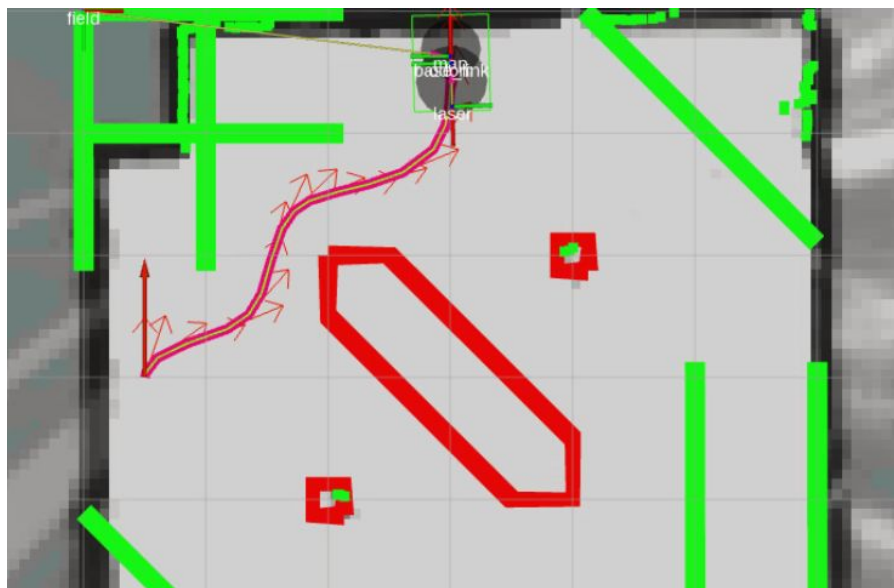
Figure 9: TEB-planned robot poses with overlaid obstacles
