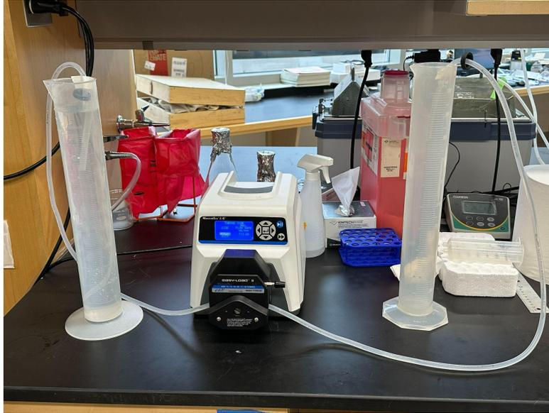
Figure 5.13: Pump calibration setup
