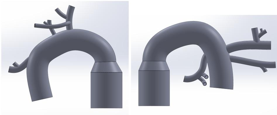
Figures 4.12 (*left*) and 4.13 (*right*): Models of left (*left*) and right (*right*) pneumonectomy assemblies in SOLIDWORKS.
