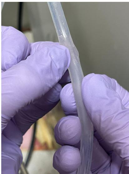
Figure 5.17: Crack formed in tubing where it ran through the peristaltic pump. This crack formed over the course of a 48 hour flow test.
