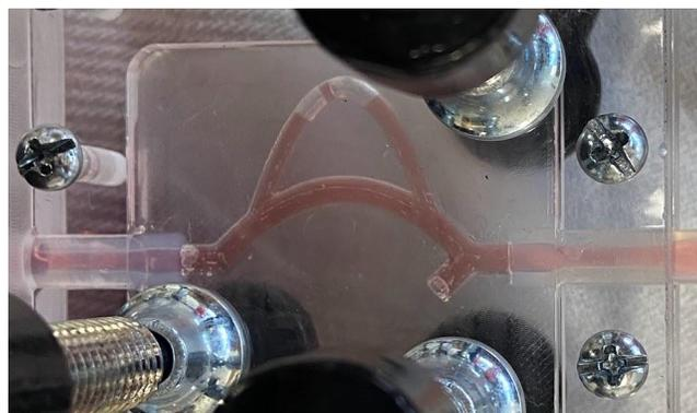
Figure 4.36 : Air bubbles formed in a smaller vessel in the pneumonectomy vasculature model during fluid flow testing.
