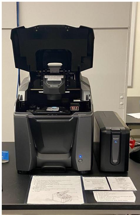
Figure 5.19 : Keyence BZ-X Fluorescence Microscope with a PDMS sample loaded inside.
