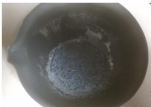
Fig. 39: Zinc Acetate After Decomposition (Note: Produced smoke blackened the crucible)
