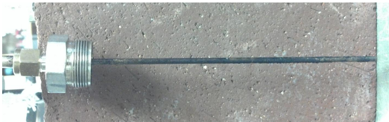
Fig. 26: The Gas Inlet Line
