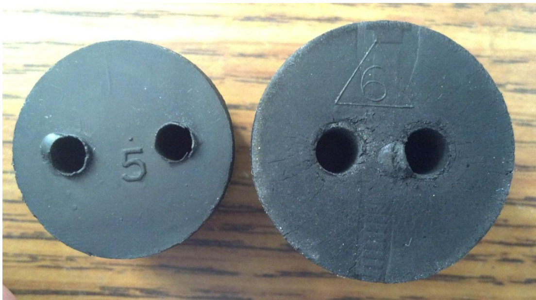
Fig 62: The visible wear and tear from usage of the rubber stoppers.
