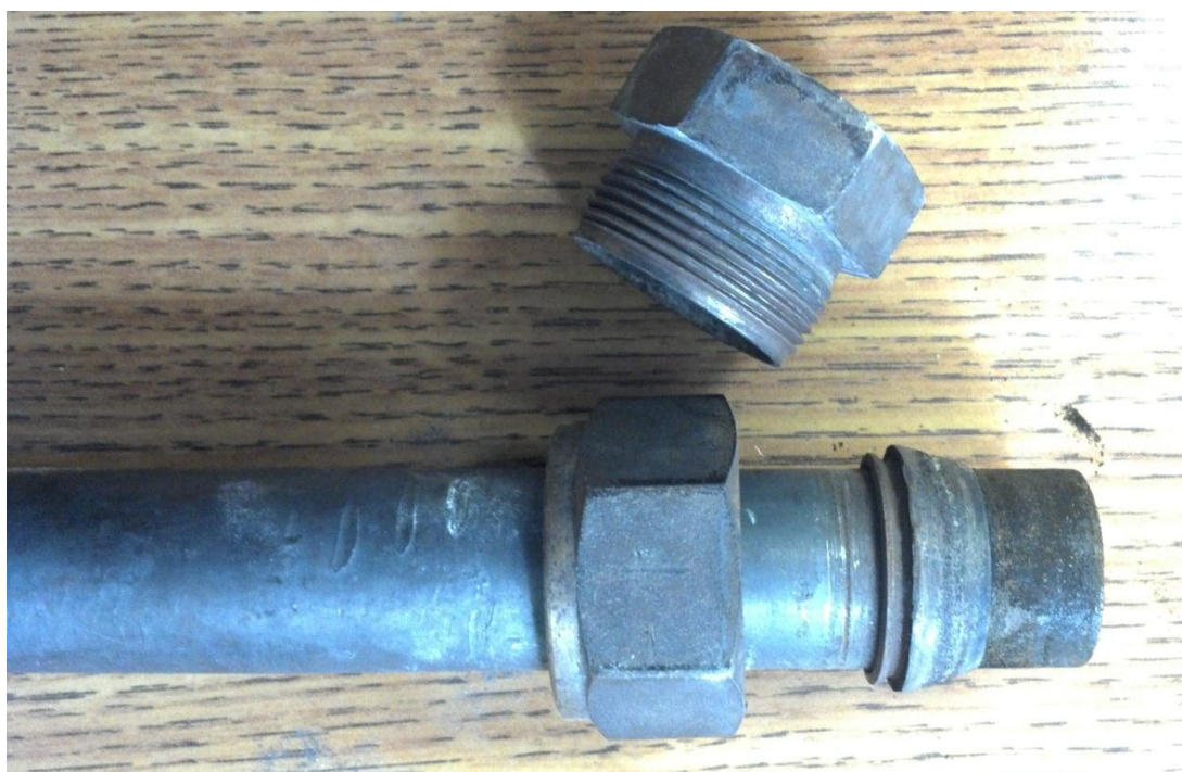
Fig 61: The bottom face of the reactor tube after the completion of experimental runs
