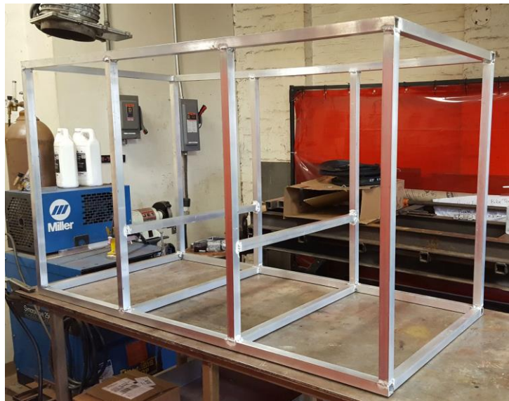
Figure 6: The Housing Box Welded in Washburn Manufacturing Labs (Photo by Cameron Hastings)
