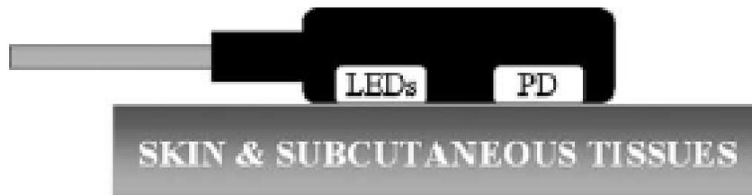
Figure 2.4: Reflectance pulse oximetry
