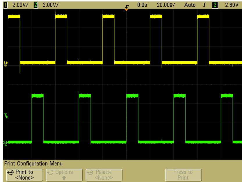
**Figure 6.4:LED driver timing diagram with 2.5ms time increments**
