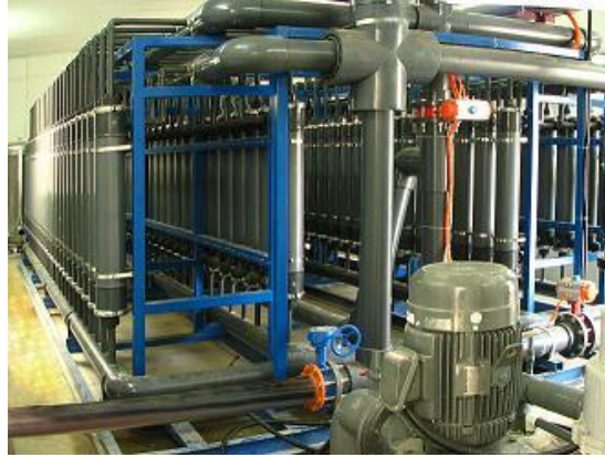
Figure 8: A spirally wound UF membrane system (24: trade gateway)
