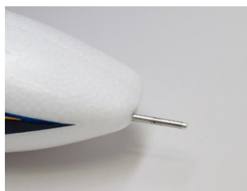
Figure 30 Pitot tube assembled at nose of UAV [12].
