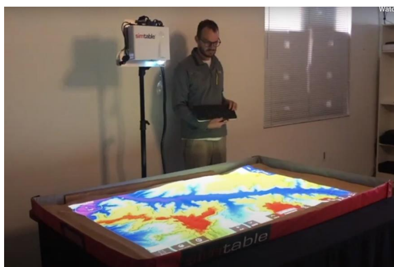
Figure 5: Simtable Sandtable with Projector and Camera (Simtable n.d.-a)
