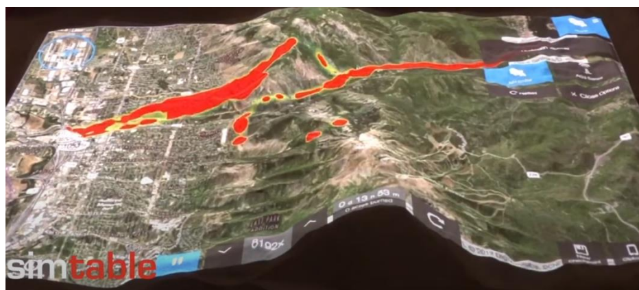
Figure 9: Simtable Smoke Plume Simulation with Smoke Cresting a Mountain due to Wind (simtablevideos 2022)
