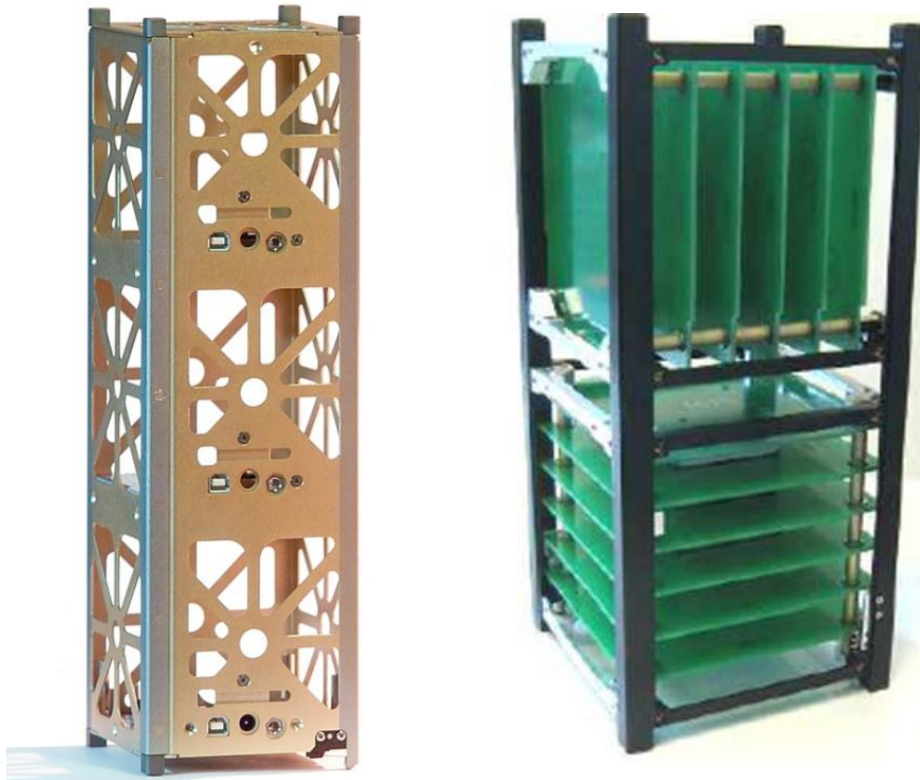
Figure 10 – CubeSat structure provided by the CubeSat Kit (left) [9] for a 3U model and by ISIS [7] for a 2U model
