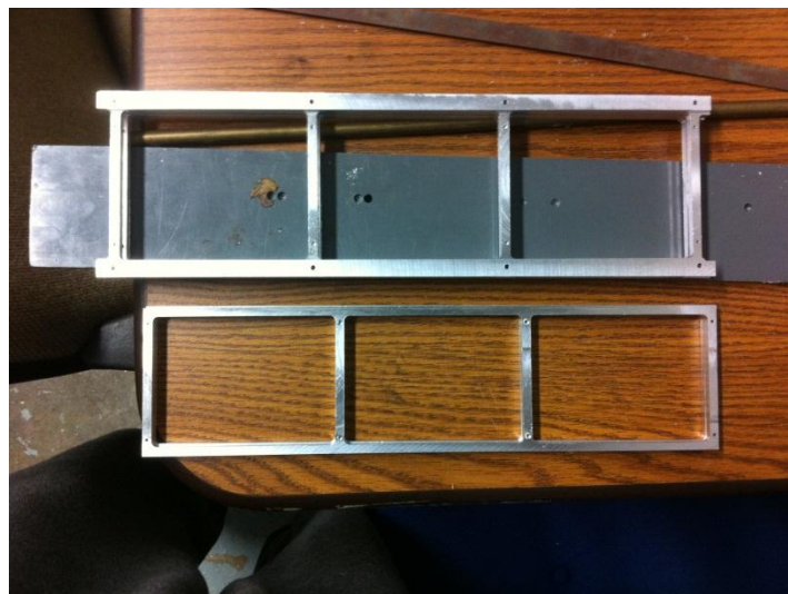
Figure 19 – Completed Railed & Connecting Panels [51]
