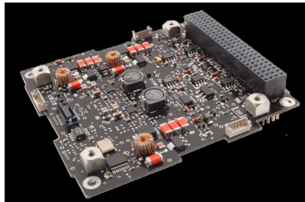
Figure 5 – Flight-Ready PMAD from Clyde Space [35]
