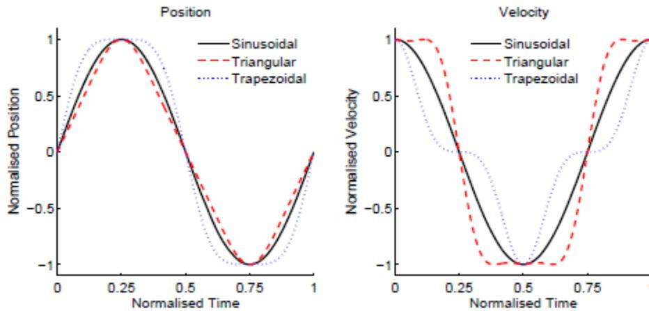
Figure 10: Position and Velocity Plots for the Tested Flapping Motions [Copyright: IEEE Robotics and Automation]
