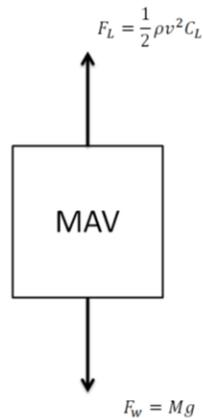
Figure 16: Free-Body Diagram in the Z-Direction (Involving Lift and Weight)
