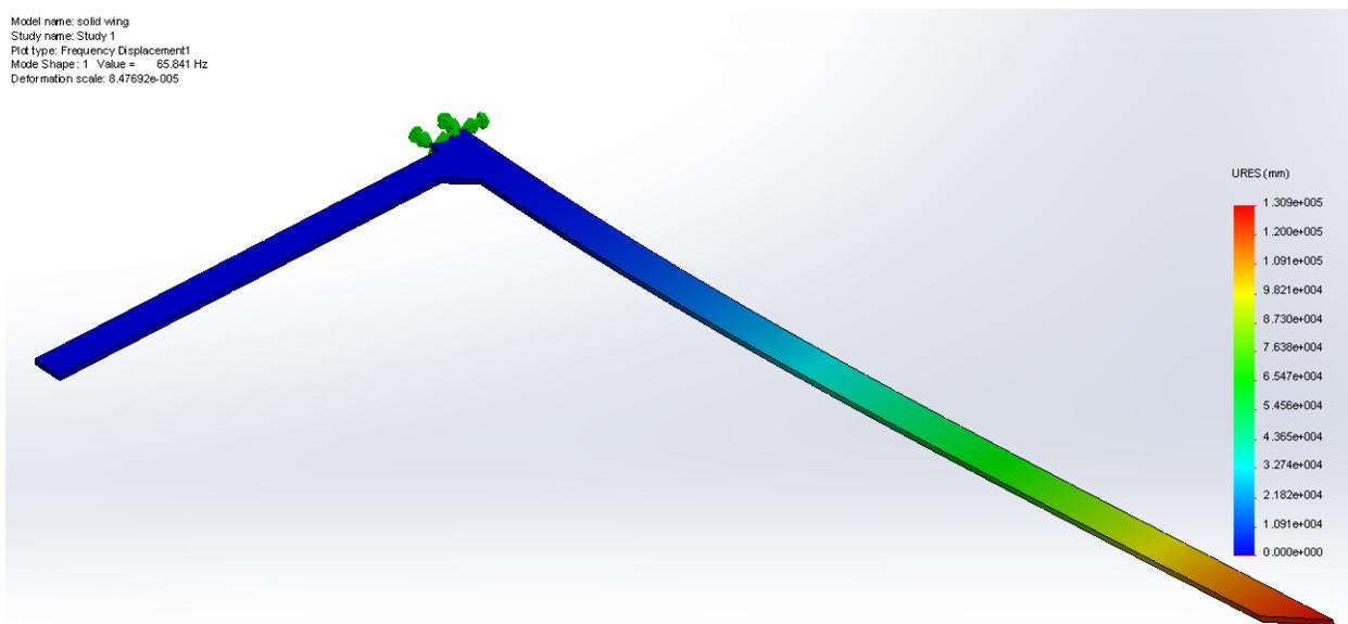
Figure 24: Wing Spar Vibration Testing in SolidWorks
