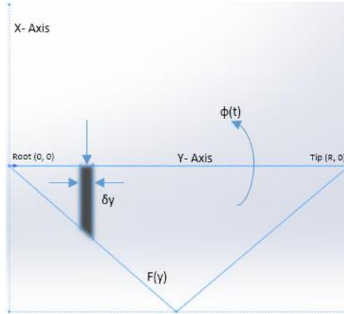
Figure 8: Differential Wing Blade Analysis
