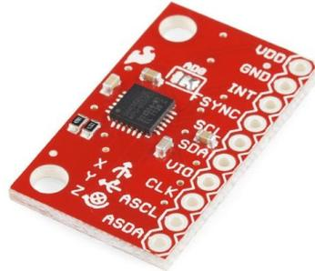
Figure 21: MPU-6050 IMU [Copyright: SparkFun Inc.]
