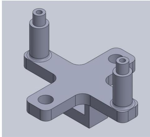
**Figure 12: SolidWorks Isometric View of the Chassis**
