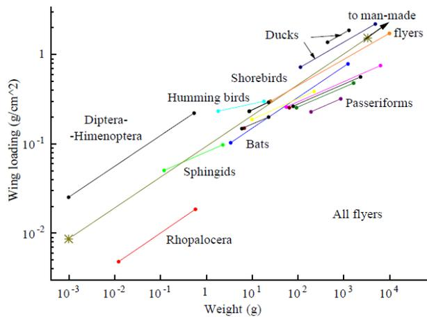
Figure 3: Wing Loading vs. Weight for Variety of Birds
