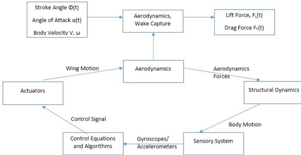
Figure 5: In-depth Systematic Flowchart to Fulfill Motion
