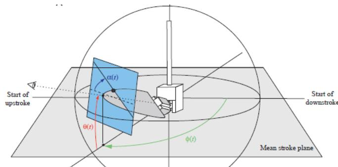
Figure 2: Wing Position defined by the Stroke Angle, Elevation angle and Angle of Attack
