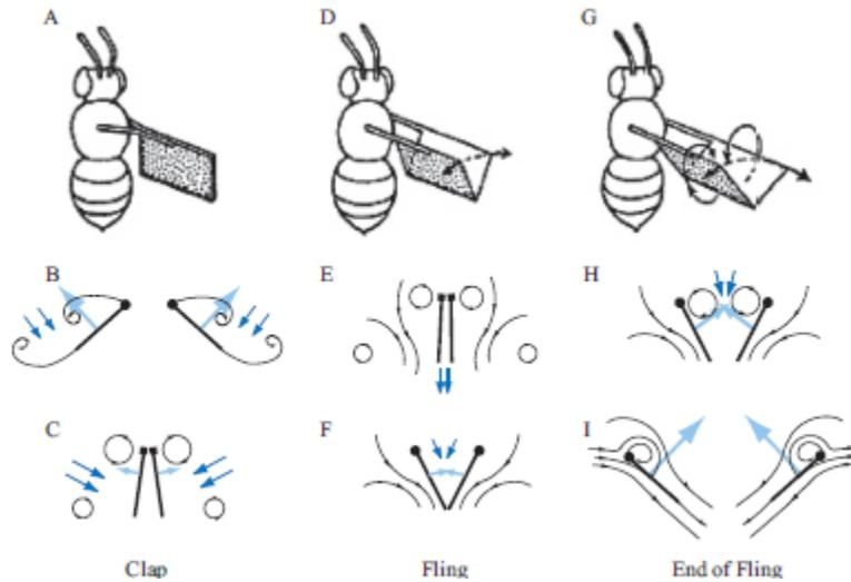
Figure 6: Clap and Fling Mechanism [23]
