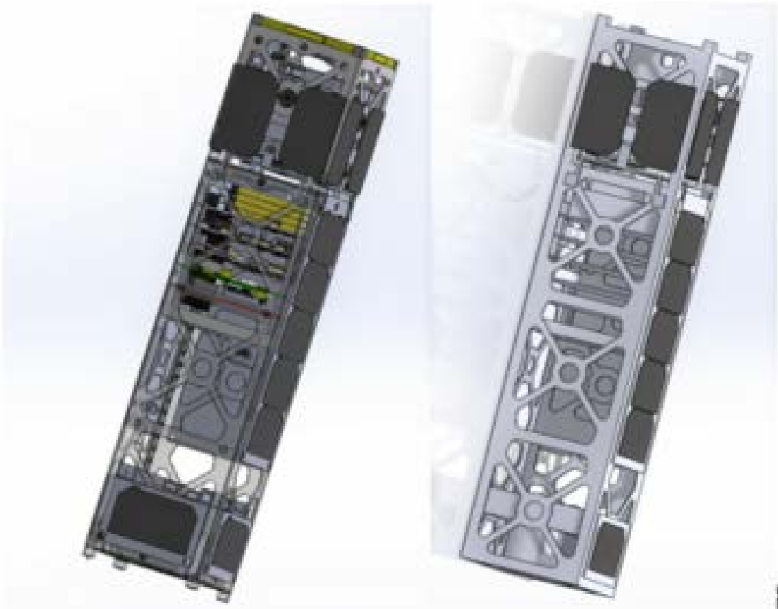
Figure 17: The de-featured 4U CubeSat COMSOL model compared to the unaltered model.
