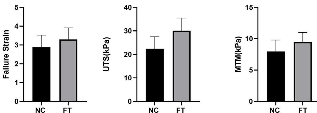
**Figure 16: Bar graphs comparing mechanical values of NC and FT tissue rings. Values are expressed as means  $\pm$  SD (n of NC = 11, n of FT = 15). Failure strain (left; NC =  $2.88 \pm 0.644$ , FT =  $3.30 \pm 0.609$ ), ultimate tensile stress (middle; NC =  $22.4 \pm 5.09$ , FT =  $30.2 \pm 5.32$ ) and MTM (right; NC =  $7.98 \pm 1.82$ , FT =  $9.50 \pm 1.51$ ) of NC and FT tissue rings**
