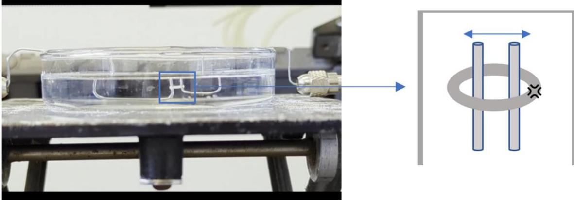
**Figure 7: Tissue Ring mounted onto custom sample wires prior to sample being stretched until failure**
