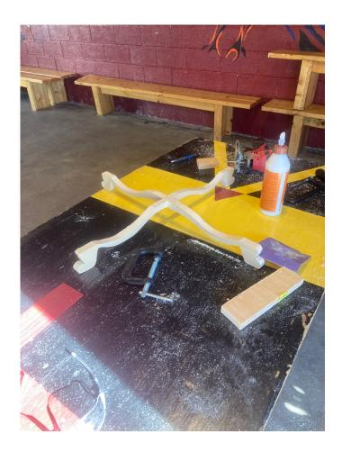
The solution to this was to use oak. A saber saw was used to cut hard oak into the shape of legs. The circular wood sections of track are going to be produced in a similar fashion. The metal frame is made out of 16 gauge mild steel sheet metal, with the intention being to tack weld the pieces together. The parts are pictured on the next page.
