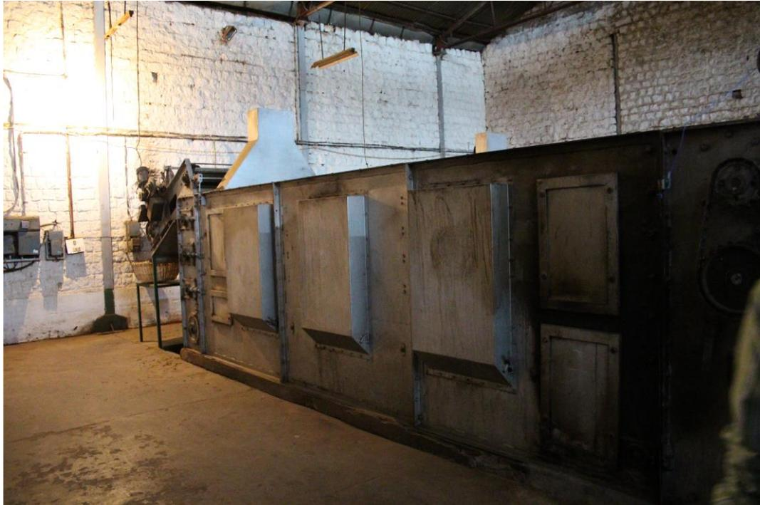
*Factories used large capacity dryers fuelled by wood furnaces.*
