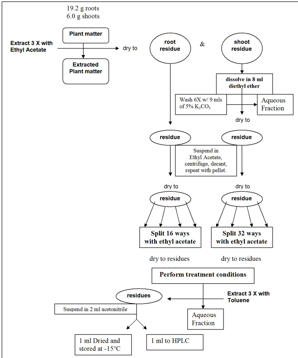
Figure 5: Flowchart depicting the preparation of hydrolysis samples.
