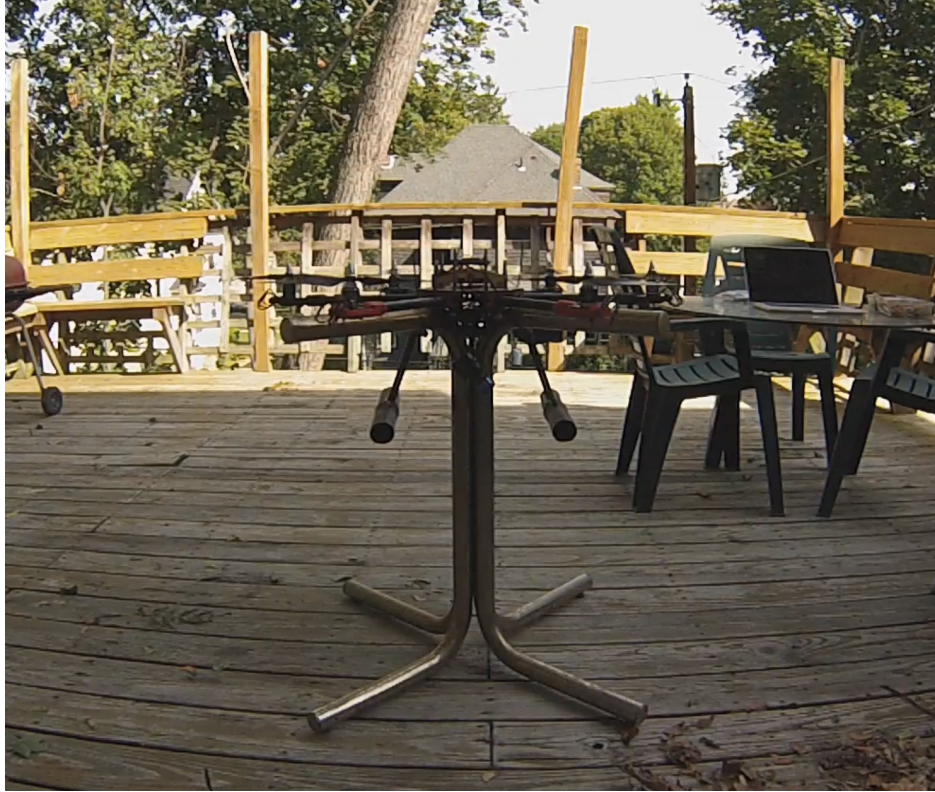
Figure 39: Drone fitness testing required strapping the system down to simulate full load on all components and sensors for calibration.
