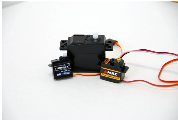
Figure 10: Servos provide rotational motion with positional awareness.
