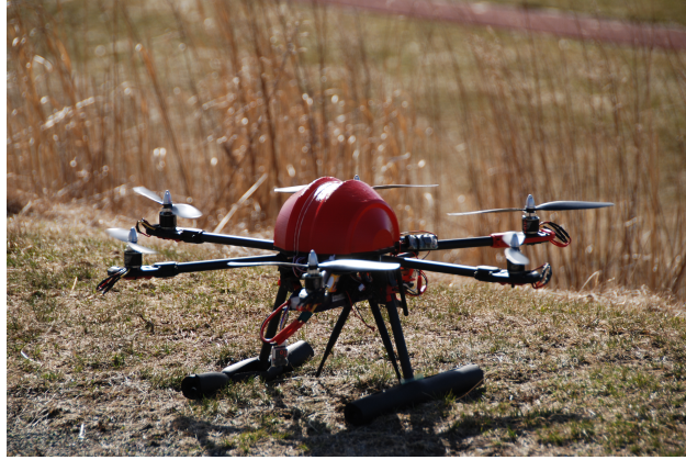
Figure 26: The Tarot 680 Pro is an easy to construct off-the-shelf hex frame solution.
