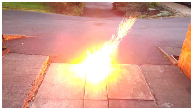
Figure 17: Lithium is explosive when exposed to moisture. Over-voltage or punctures in a LiPo cell can be catastrophic. [18]
