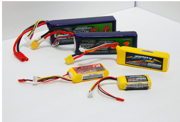
Figure 16: LiPo batteries provide high density power in a small package.
