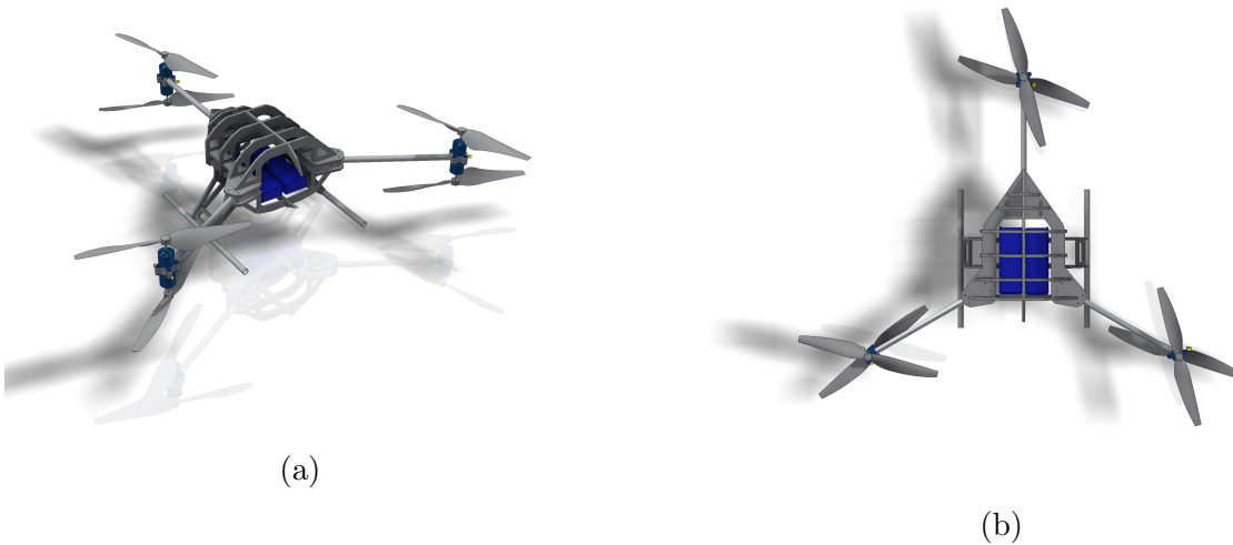
Figure 29: The Y6 Hex frame is another frame type experiment.
