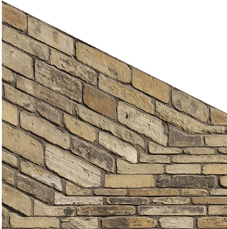
Figure 48: Construction of a quad in OpenGL is done with two separate triangles. This causes a seam to be visible when the quad is re-sized to irregular shapes.
