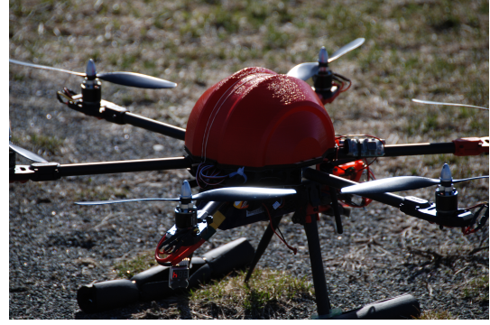
(b) Printed Electronics Hood in Red
