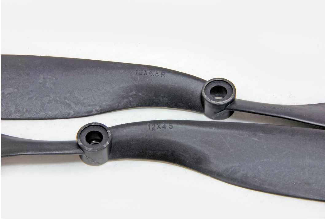
Figure 2: Each propeller has a marking indicating its diameter and pitch values. The diameter and pitch values for these propellers are 12in x 4.5in
