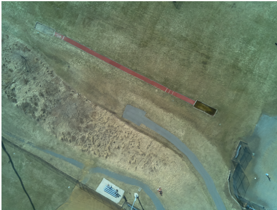
Figure 41: This picture was transmitted and received over a 1.3mile WiFi link. GPS location 42^{\circ}16'44.0'' N 71^{\circ}46'53.5'' W.
