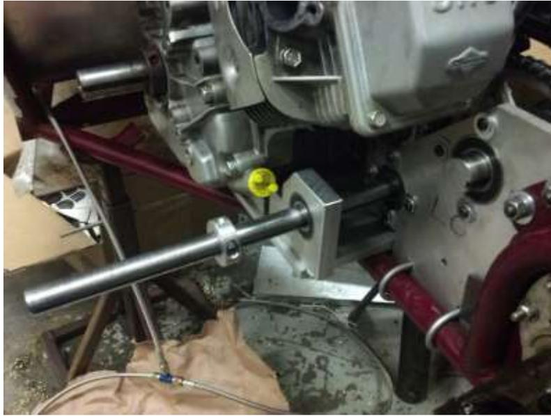
Figure 16: Mounted Support Bearing
