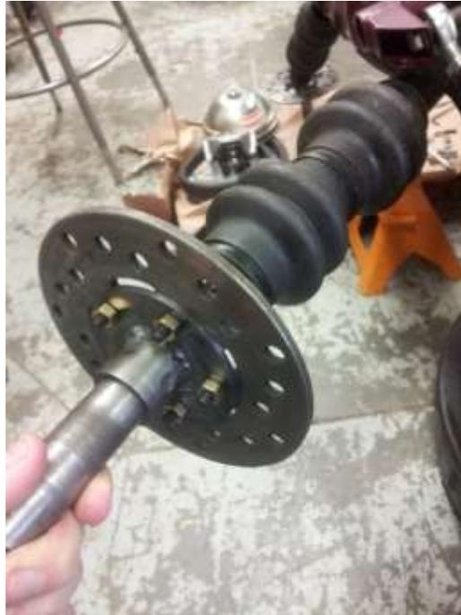
**Figure 30: Rotors Mounted to Rear Driveshaft**
