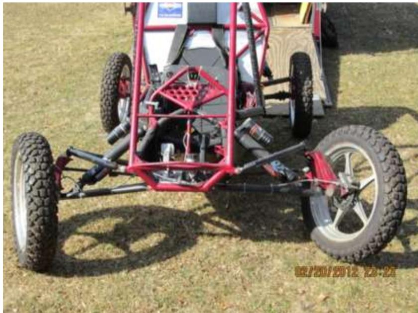
**Figure 38: Incorrect steering angles**
