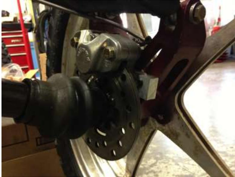
**Figure 34: Finished Rear Brake Assembly**
