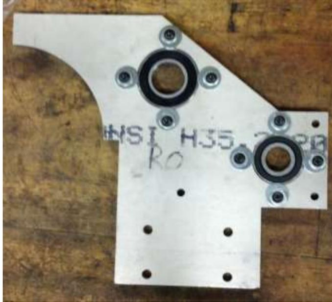
Figure 13: Finished Bearing Plate
