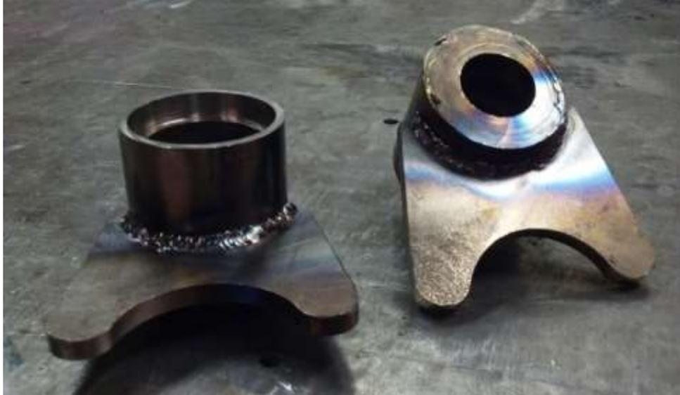
**Figure 72: Caliper Mounts Welded to Spindle Tubes**
