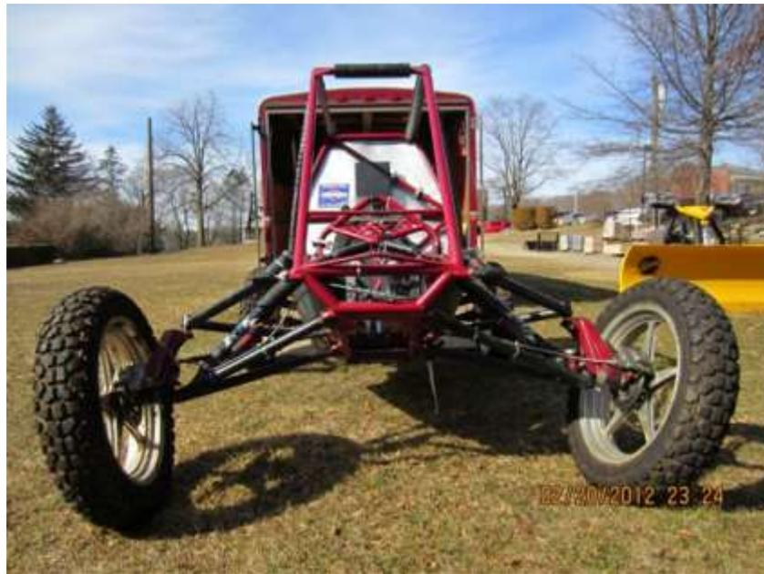
**Figure 36: Positive camber gain**
