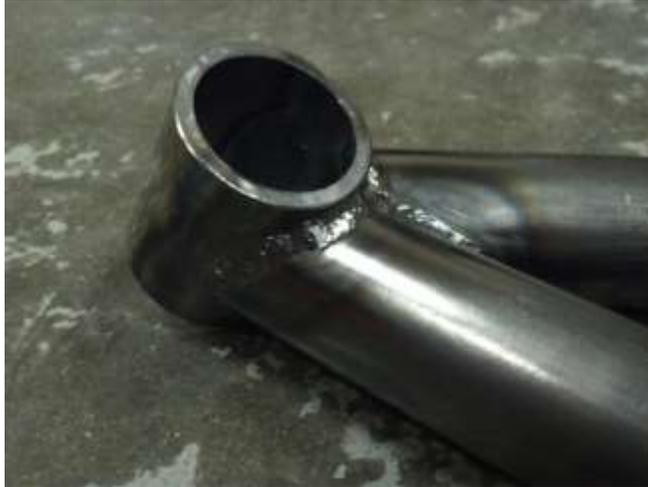
Figure 66: Ball Joint End
