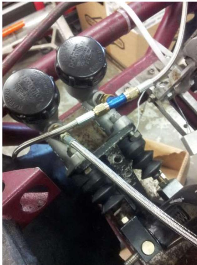
Figure 23: New Master Cylinder Setup
