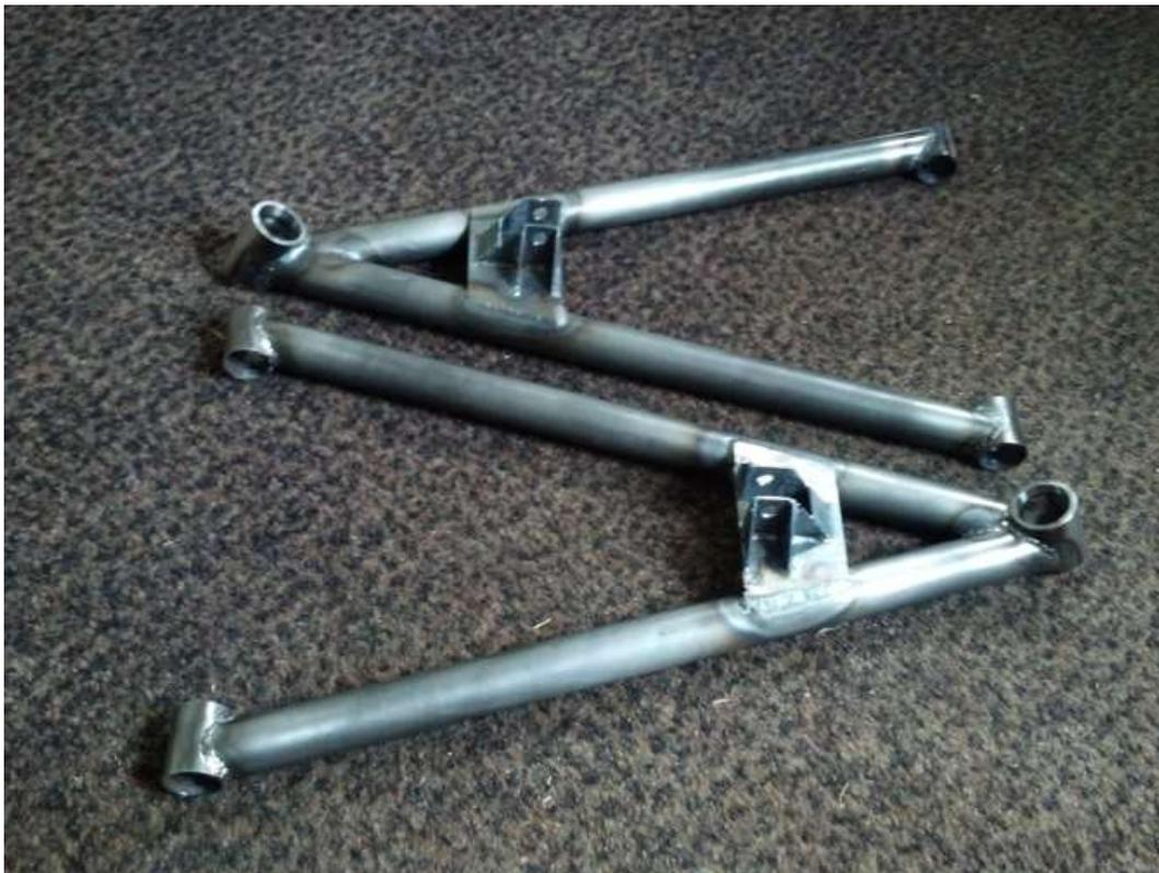
Figure 67: Lower Control Arms After Welding
