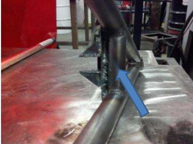
**Figure 63: Shock Mount Support Tube**
