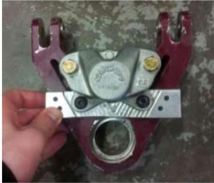
**Figure 27: Location of Caliper on Rear Knuckle**
