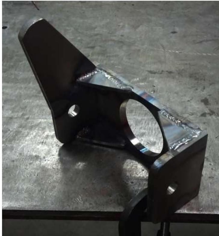
**Figure 73: Body of Knuckle Welded Together**
