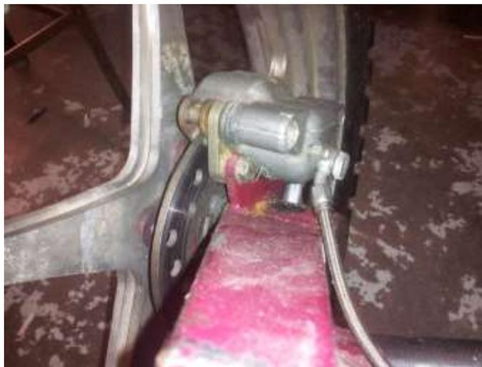
Figure 18: Original Front Brake Caliper/Rotor Orientation
