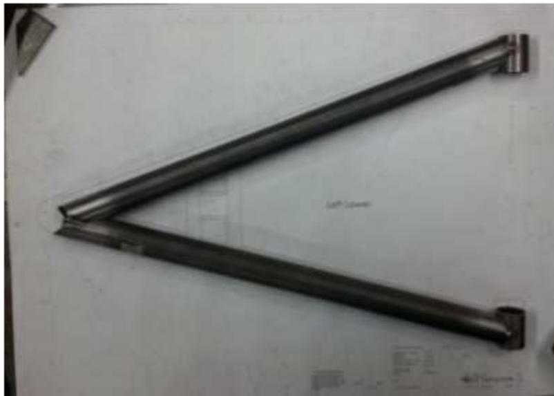
**Figure 61: Layout for Welding**
