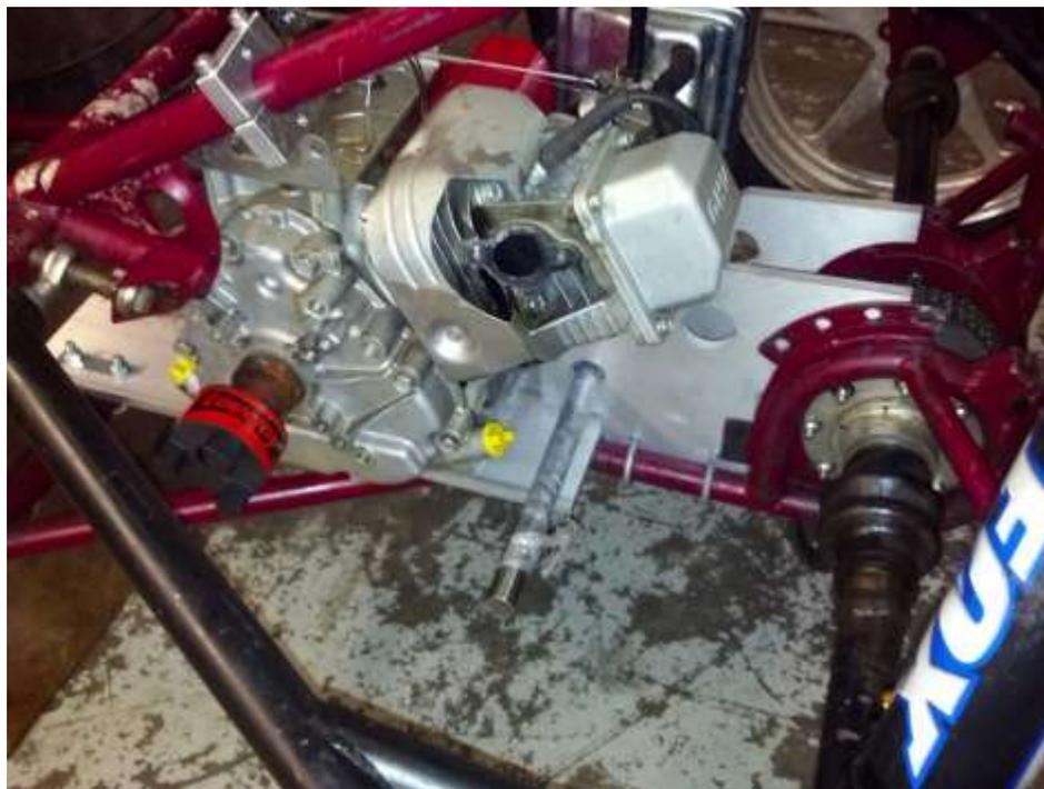
Figure 10: Engine Mounted
