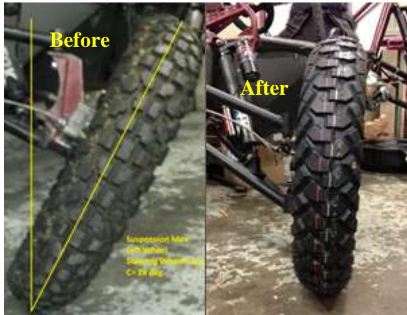
**Figure 78: Difference in Turning Camber**
