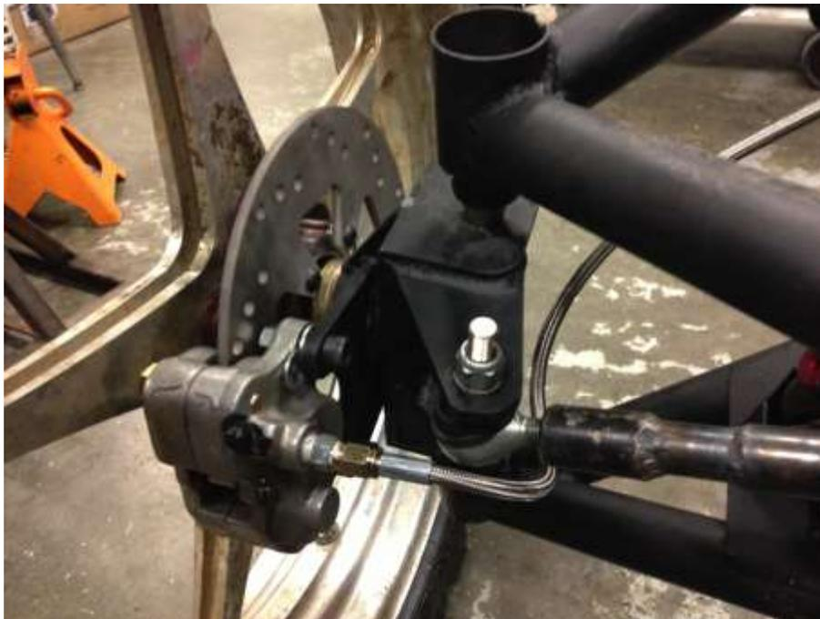
**Figure 33: Finished Front Brake Assembly**
