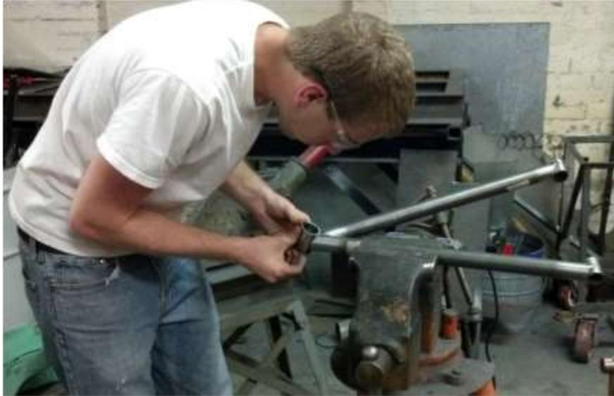
**Figure 62: Hand Grinding for Fit**
