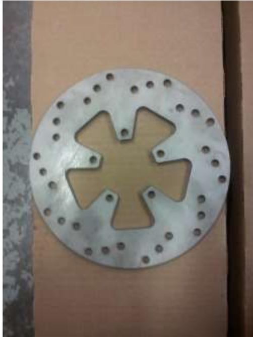
**Figure 32: Rotor after Waterjetting**
