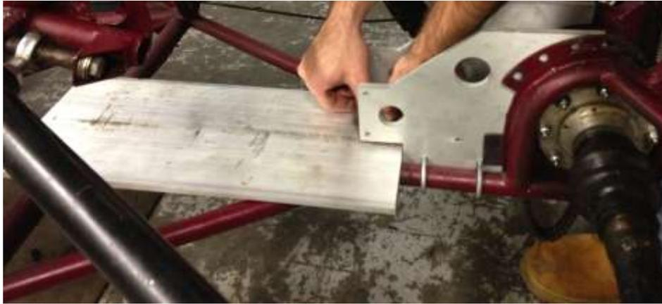
Figure 9: Mocking up the Engine Mount Plate
