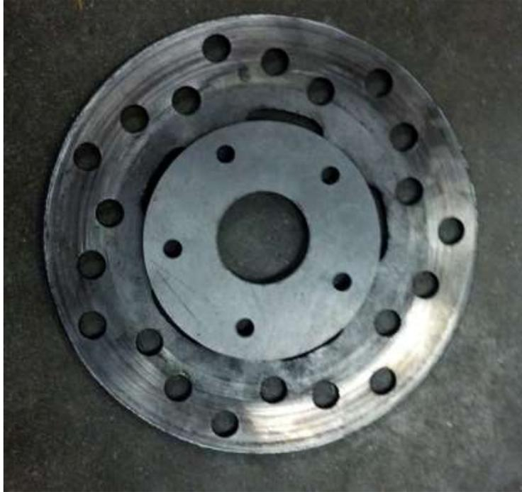
**Figure 28: Hub on Rotor**
