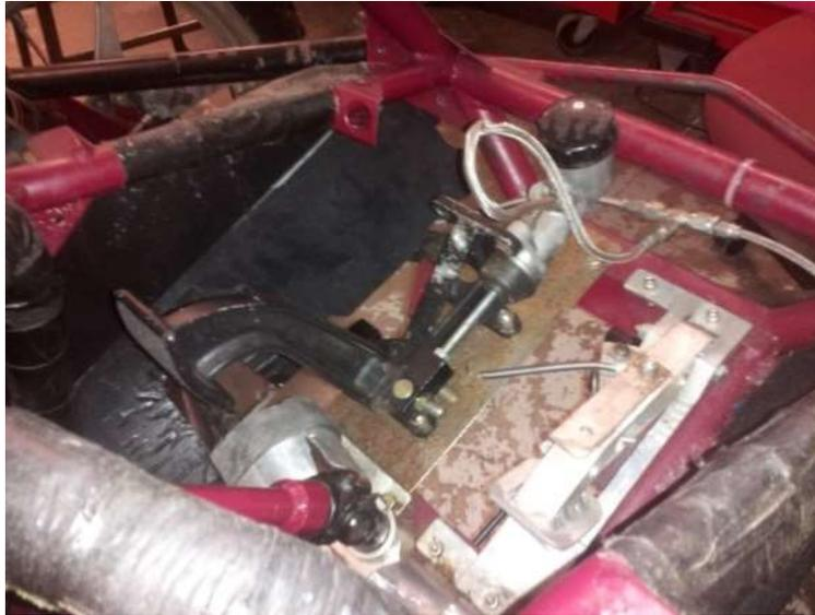
**Figure 20: Original Pedal/Master Cylinder Setup**
