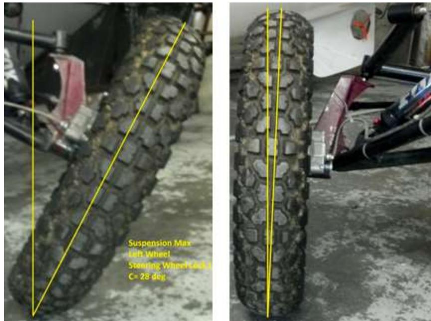
**Figure 39: Camber at max compression and full-lock left**
