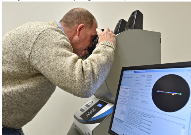
Figure 5.6: Subject being tested using the SafetyScan system. Near the top of the machine is the camera system to measure eye movement (Staples 2018)
