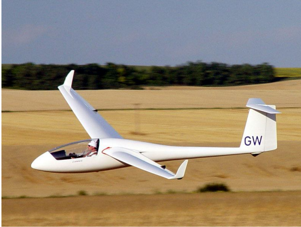
Figure 37: Winglet Designed by Steve Willits from Ref [35]
