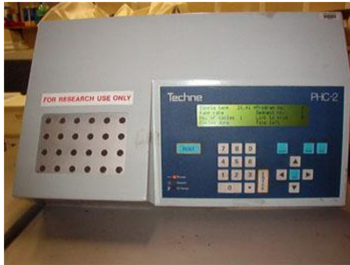
Figure-10: Picture of a Thermocycler Used for PCR. This machine is used to cycle DNA samples between alternative periods of heating (to denature DNA strands) and cooling (to allow primers to anneal to the DNA, facilitating DNA replication). This process rapidly amplifies portions of DNA between the primers, allowing DNA profiling at specific forensic loci. (Rice, 2006)
