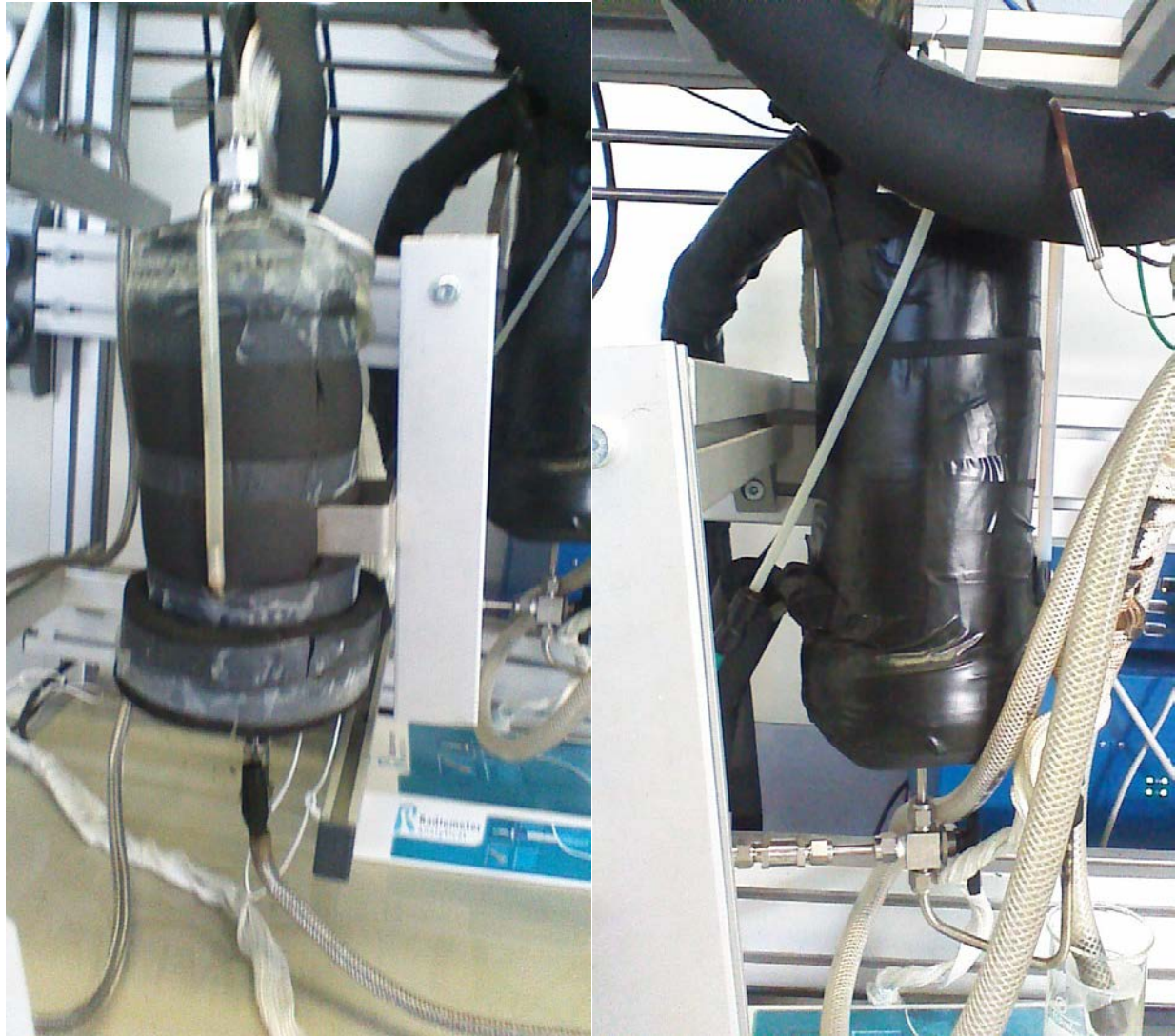
Figure 46: Air and Hydrogen humidifiers
