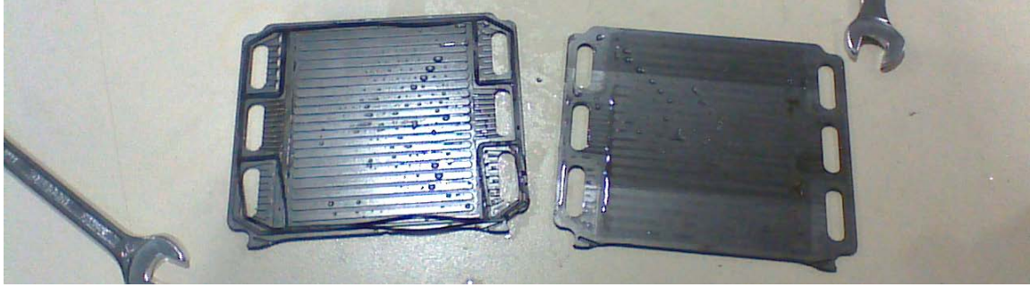
Figure 40: A bipolar plate (on left) and additional plate to protect the current collector plate.
