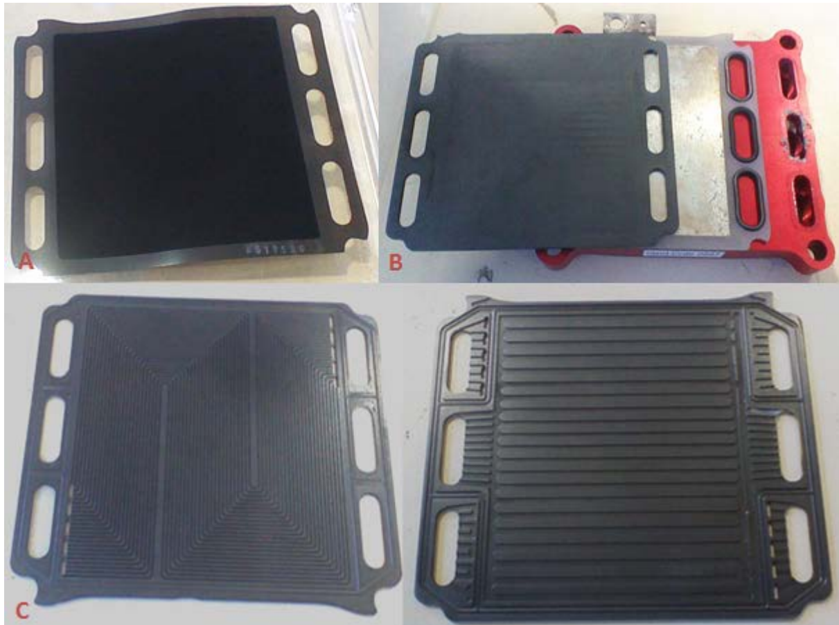
Figure 12: Parts of the fuel cell; A. Membrane-electrode assembly (MEA) used; B. Red end plate, current collecting plate and a channel plate; C. Bipolar plates in which fuel ( H_2 or Air) flows on the side with a serpentine path (left plate) and water flows on the plate with a rectangular path (right).
