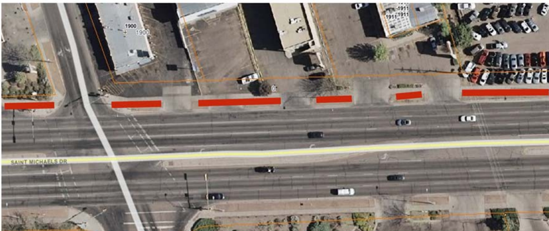
Figure 40 St. Michael's Drive with 4 Curb Cuts
