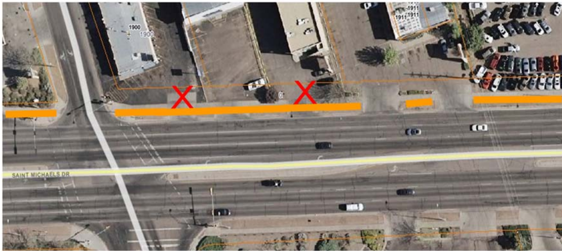
Figure 39 Crossing off 2 Curb Cuts
