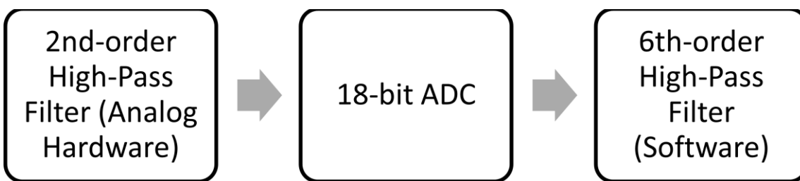
Figure 7 – Diagram of Software and Hardware Sections of the 8 th -order High Pass Filtering Using an ADC
