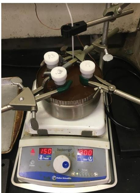
Figure 3.2.4: Oil bath Hydrolysis Setup
