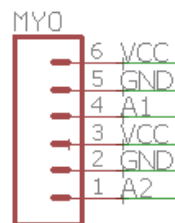
Figure 1 Myoelectric Sensor Schematic Symbol
