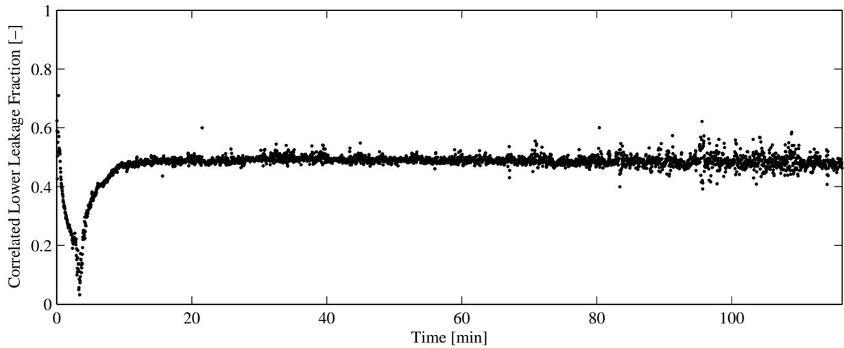
Figure G.4: Correlated lower leakage fraction for test no. 19 - Inst. #1 (HFC-125)
