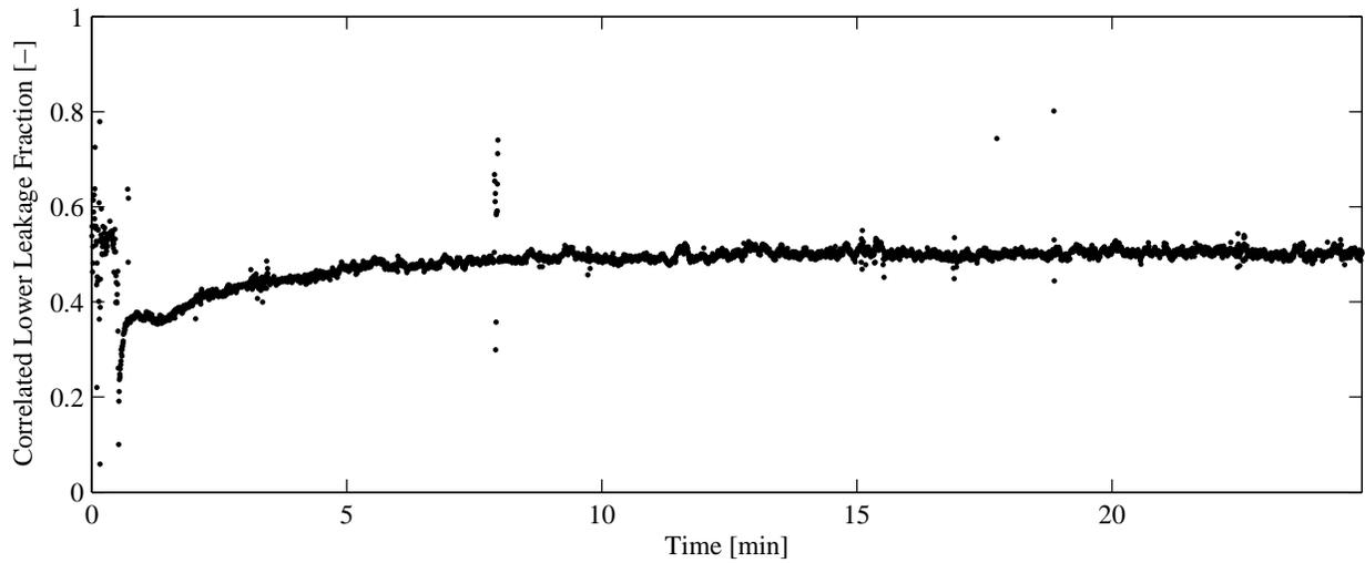
Figure G.13: Correlated lower leakage fraction for test no. 29 - Inst. #1 (HFC-23)
