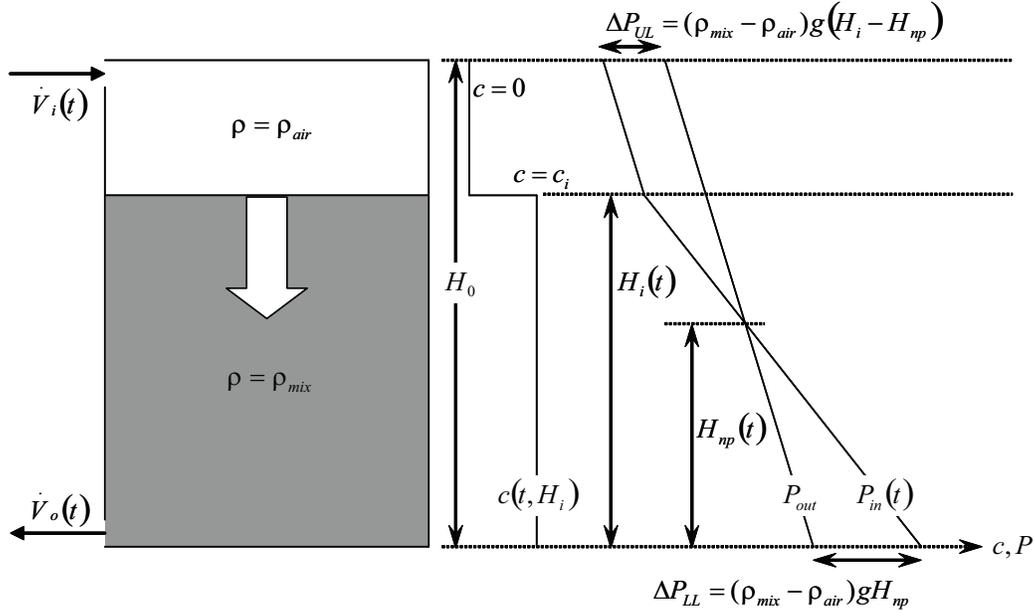
Figure 2.1: Sharp descending interface hydrostatic pressure profile. As shown in the figure, a sharp interface forms between inflowing fresh air and the agent-air mixture.
