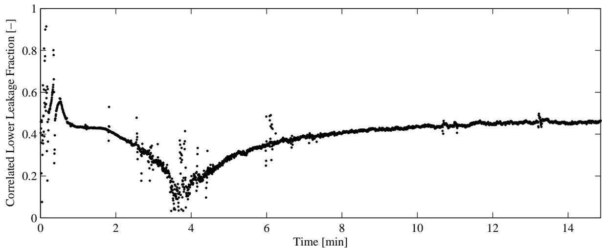
Figure G.12: Correlated lower leakage fraction for test no. 25 - Inst. #2 (HFC-227ea)
