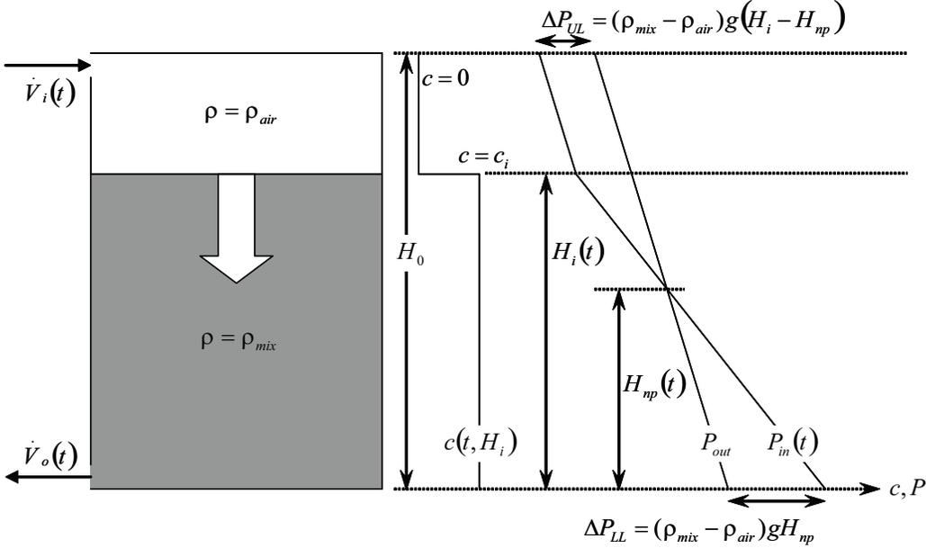
Figure B.1: Sharp interface hydrostatic pressure profile schematic
