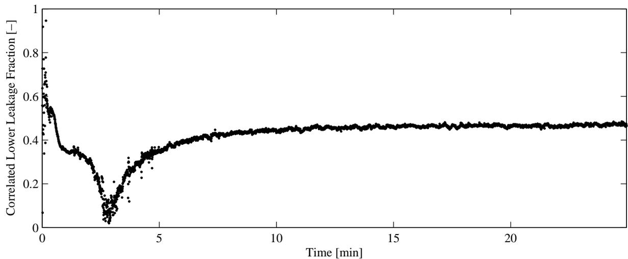
Figure G.9: Correlated lower leakage fraction for test no. 23 - Inst. #1 (HFC-227ea)
