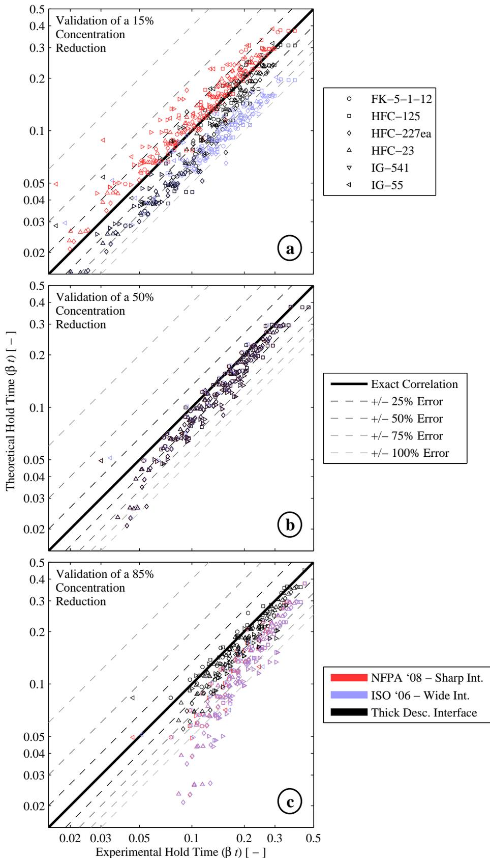
Figure J.7: The predicted theoretical hold time at 15%, 50%, and 85% concentration reduction thresholds, evaluated at any elevation, compared to the observed behavior of all clean agent types tested (pure N<sub>2</sub> not included).
