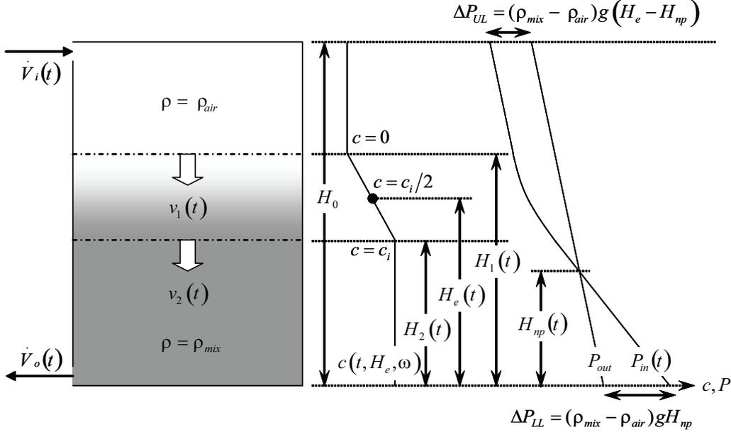
Figure B.3: Thick interface hydrostatic pressure profile schematic
