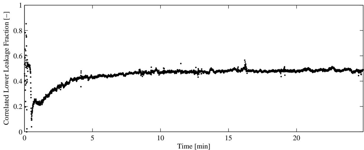
Figure G.15: Correlated lower leakage fraction for test no. 31 - Inst. #1 (HFC-23)
