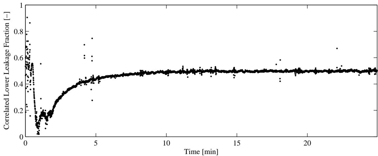
Figure G.8: Correlated lower leakage fraction for test no. 22 - Inst. #2 (HFC-227ea)
