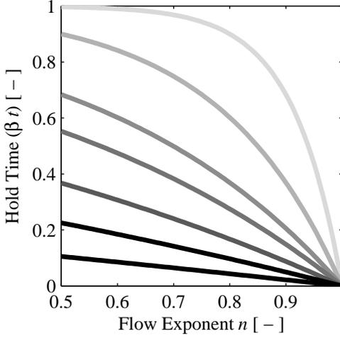
Figure B.4: Dimensionless hold time versus the flow exponent,  $n$ , for set values of the dimensionless interface height,  $\tilde{H}$  (value ranges from 0.8 towards 0 as the shade lightens).
