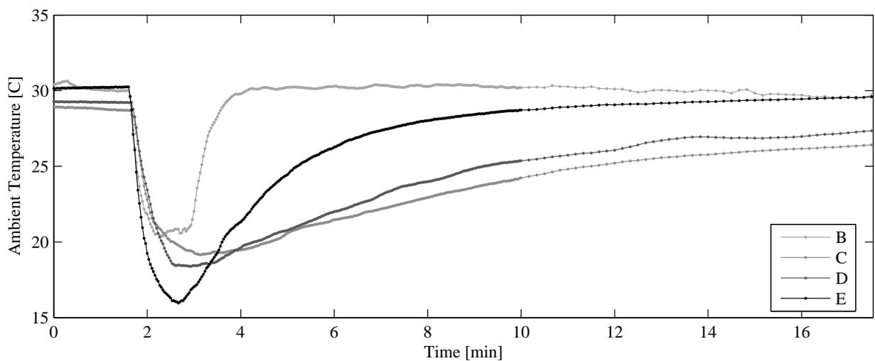
Figure F.24: Ambient temperature data for test no. 32 (IG-55)
