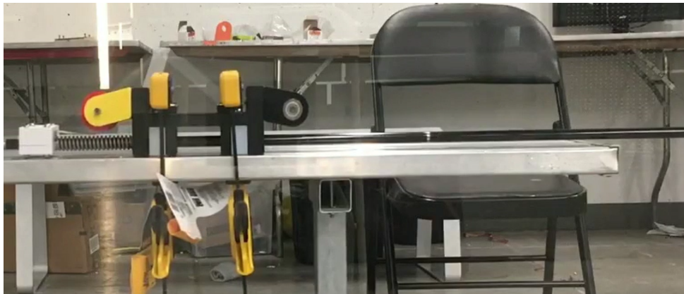
Figure 41: Newly Printed Constant Force Spring Holder
