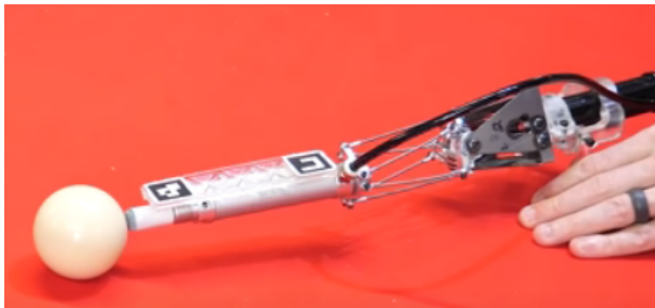
Figure 66: Automatic Pool Stick Utilizing Stuart Platform (Wighton, 2021)
