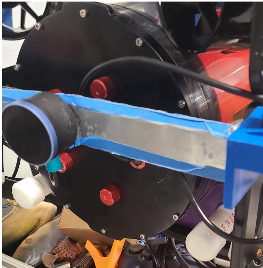
Figure 57: Front view of the installed weights system
