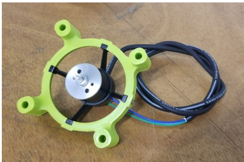
Figure 70: Motor and Motor Mount Assembly
