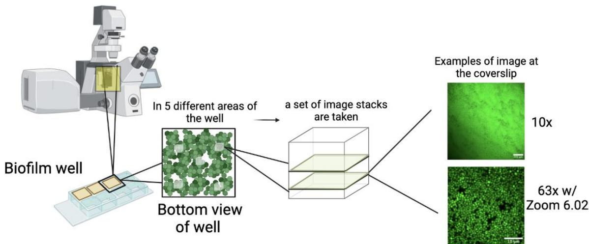
**Figure 10. Schematic of the workflow for imaging biofilms using the CLSM.**
