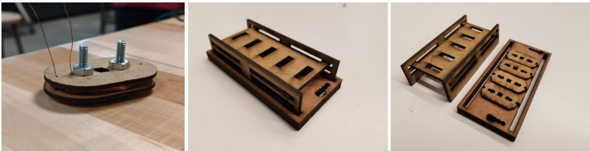
Figure 22: Shear Racetrack Fabrication (Right: large coil, Middle and Left: slide framework)
