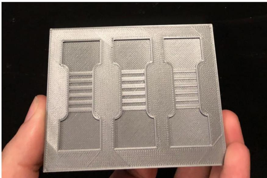
*Figure 5 3D Printed Ribbed Dog Bone Structure Mold*
