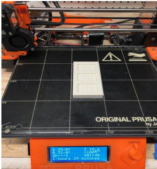
Figure 3 Prusa 3D Printer with ribbed substrate mold
