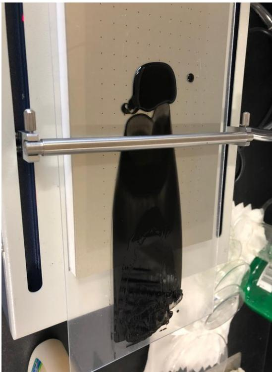
Figure 4 Automatic film coater Casting PVDF nanocomposite
