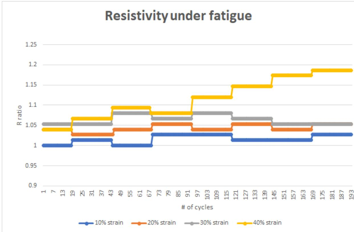
Figure 18 Graph of Resistivity under Fatigue
