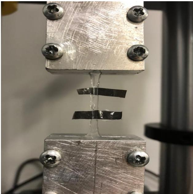
Figure 12 Elongation at 35% Divided Battery Structure
