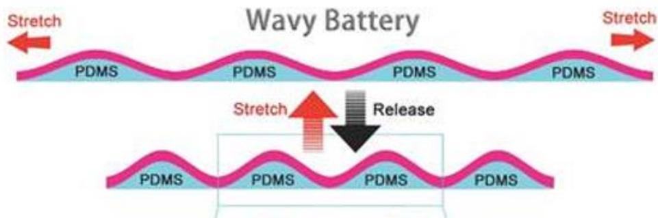
Figure 1. Buckling Example
