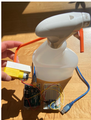
Figure 48: Automated Spray Bottle System using an Arduino Uno
