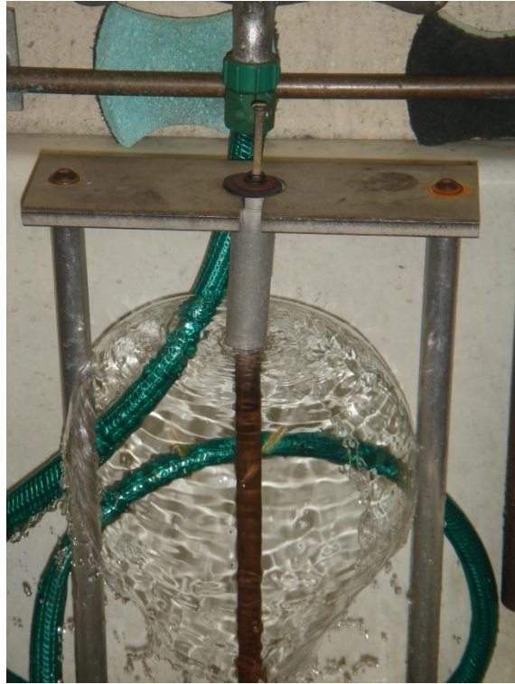
Figure 1: Jominy End Quench (JEQ) apparatus
